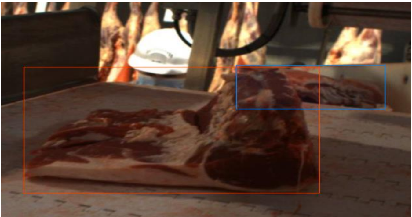
Figure 13: Image gmp_20210810_114108_9Z8j.png has two objects annotated - one naked_rack (blue rectangle) and one naked_loin (red rectangle).
