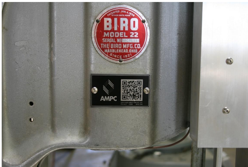
Fig 6 More than the traditional nameplate (above), the slate (below) offers a comparatively infinite array of information accessible through the cloud
