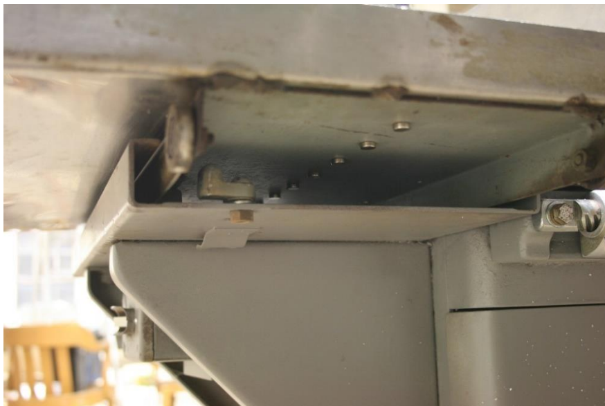
Fig 17 Neodymium magnets mounted at even intervals to the underside of meat carriage assembly.
