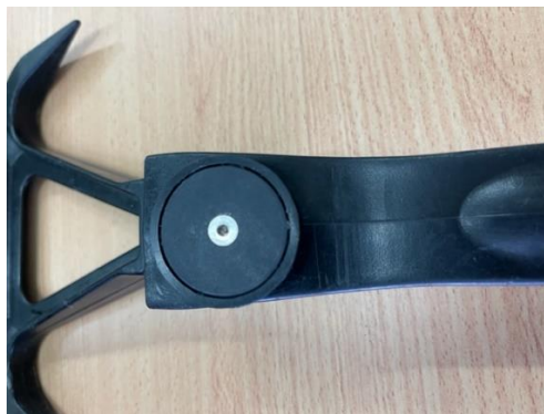
The second attempt RFID tag attached to gambrel, pictured below.
