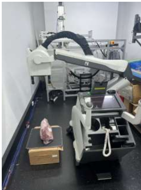
Figure 7: Micro-X Rover Mobile X-ray Cart Set up with Beef Loin
