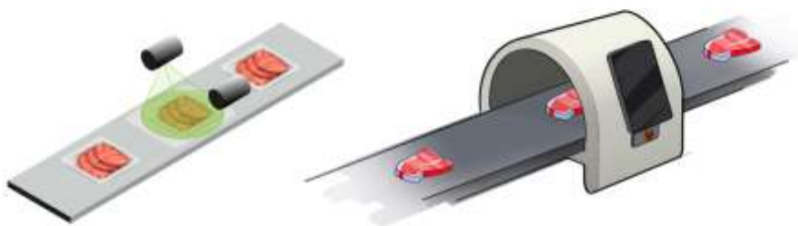
Figure 2 Flat Scanning with Multiple Sources
