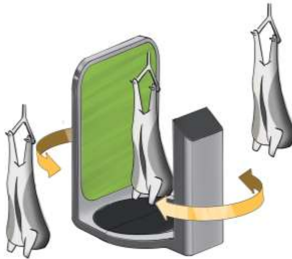
Figure 1 Rotating Scanner Concept
