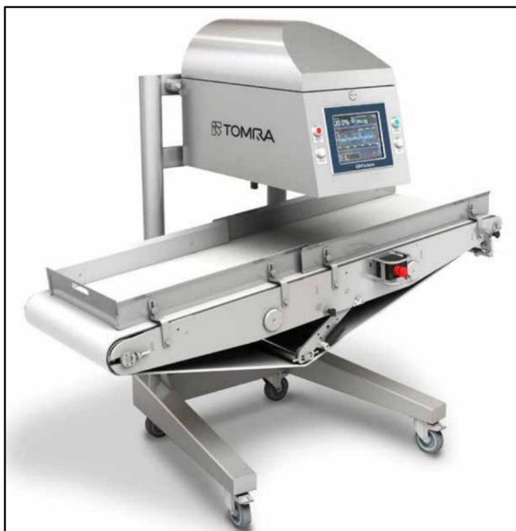
Figure 18: Standalone QVision system for processing 30 tons per hour. L: 2,900 mm, W: x 1,115 mm, H: 1,910 mm. Power draw: 0.5 kW, Compressed air: 50 L/min.
