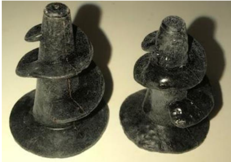
Figure 17: Sheep plug at ambient storage (left) and after exposure to 160 °C heat. The plug did not melt; however, the device was highly brittle and dry.
