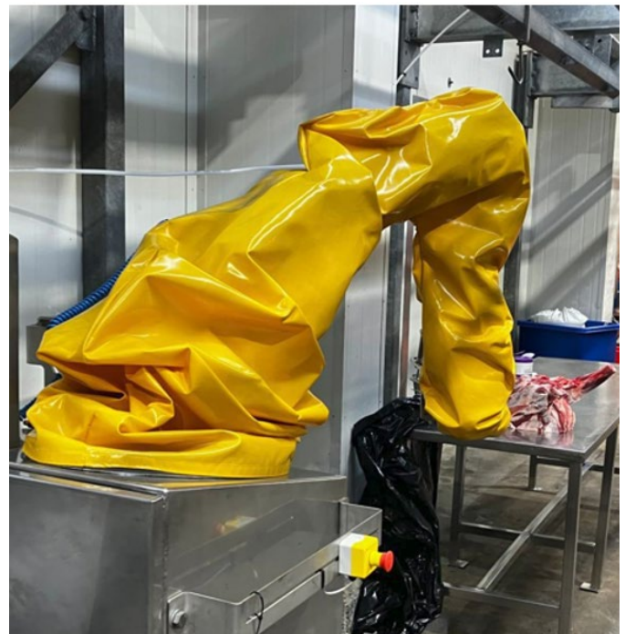
World first integrated robot unit for forequarter ribcage separation, deboning of lamb shoulders.
