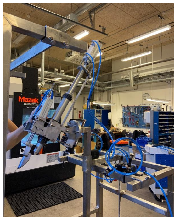
Figure 9: Adjustments of equipment at the DMRI workshop prior to shipping to Australia. Note the curved punch knife as part of the process.
