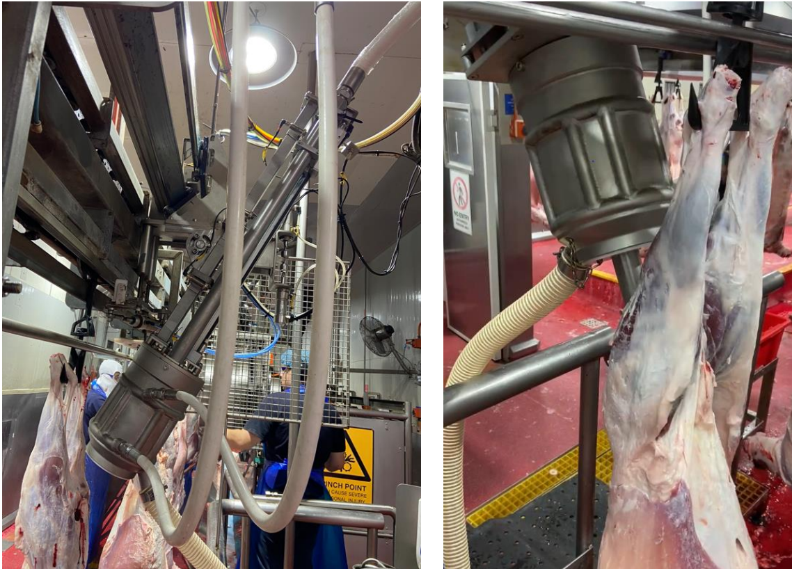
Figure 7: Rebuilt and remounted bung handler unit adapted for lamb slaughter
