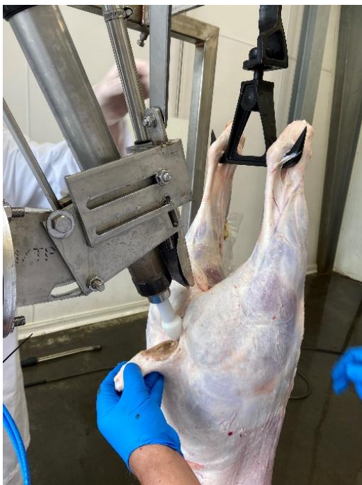
Figure 8: Insertion of cone-shaped plug during testing at the Danish slaughterhouse.
