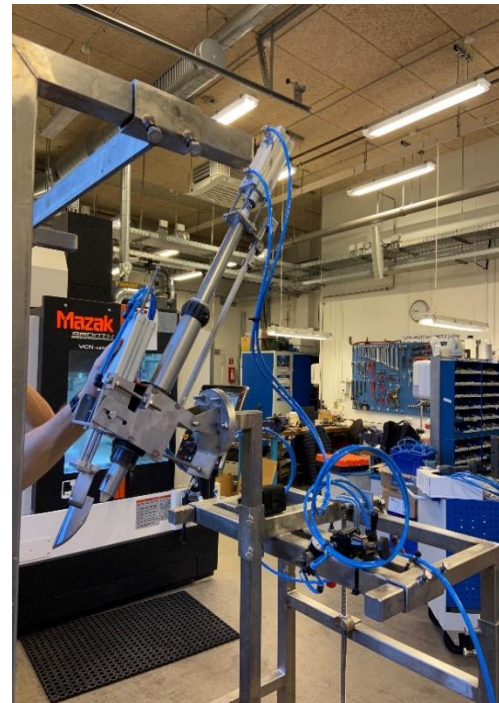
Figure 2: The semi-automatic bung cutting tool (B)
