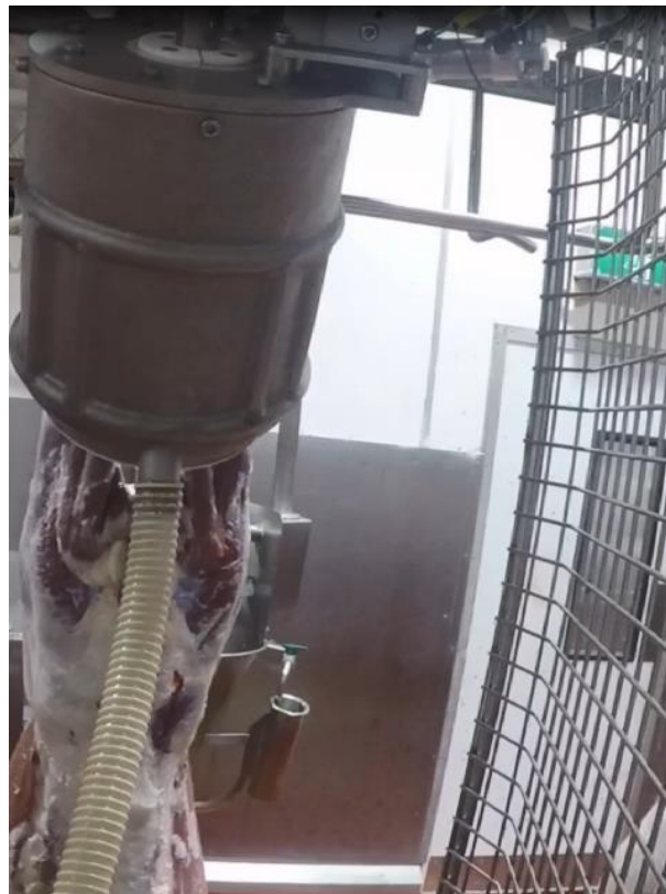
Figure 5: Commissioning the bung handler at the host site in Australia
