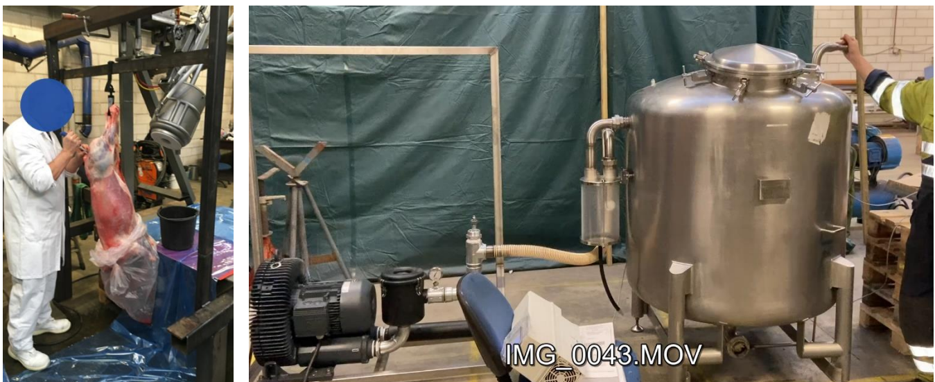
Figure 4: Cutting free the bung manually prior to initial workshop test with the bung handler prototype (left). Pump and tank components providing the controlled vacuum for the process (right)
