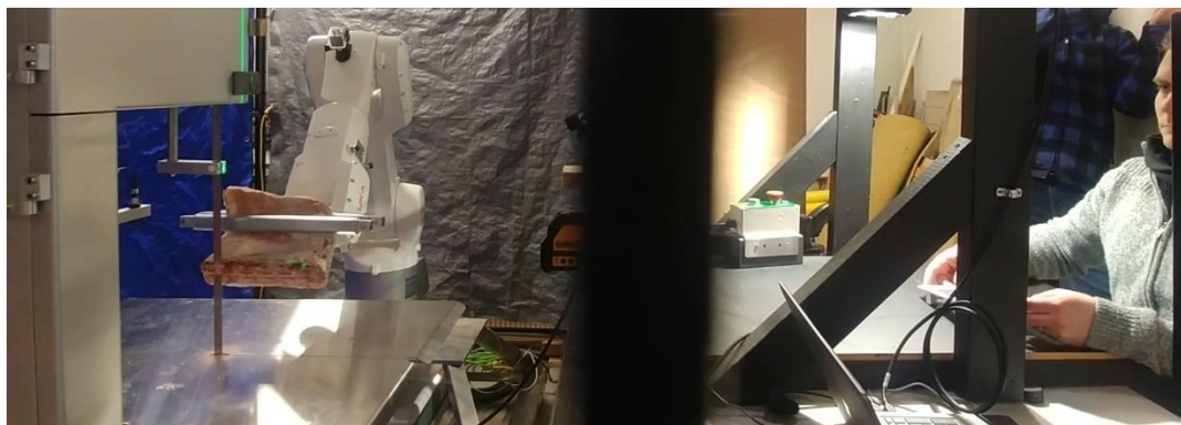
Figure 2: Photograph showing demonstration of remote chine bone cutting.
