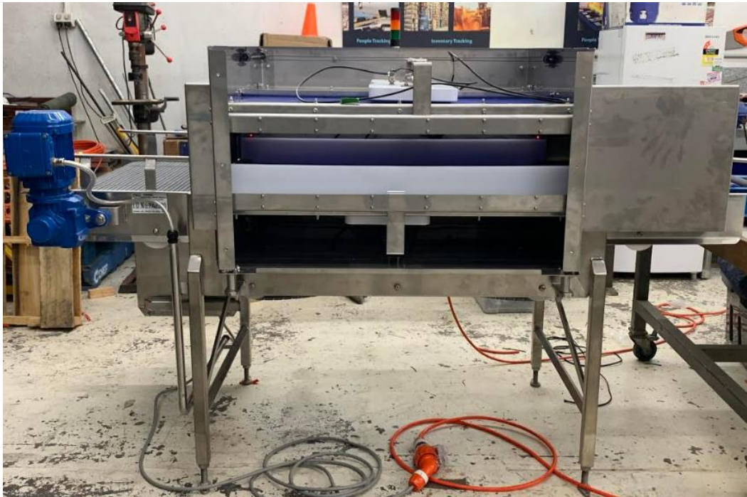
Figure 5: RFID Tunnel and conveyor – side view – Tunnel cover panel removed.
