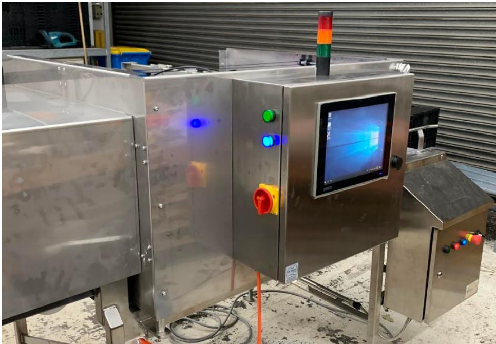
Figure 7: RFID Tunnel and conveyor – Electronics cabinet and display
