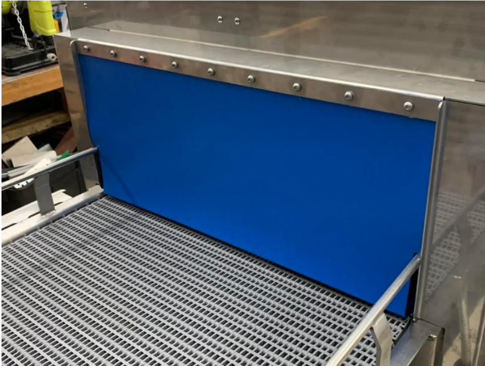
Figure 9: RFID Tunnel and conveyor – RF Shielding Curtain
