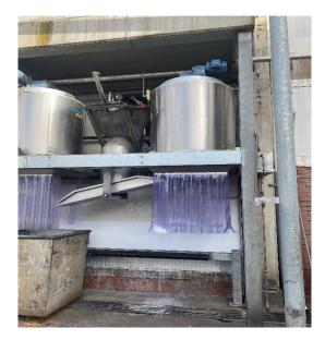
This photo shows the second ice machine in position. Modifications have also been made to the hide chute to allow it to swivel between the two hide bins like a seesaw. A laser has been installed on each ice machine that is triggered when the corresponding hide bin reaches its capacity which will trigger the chute to swivel to the other hide bin to begin filling. The chute can also be manually switched if necessary.
