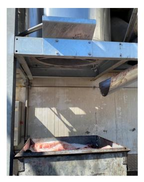
This photo shows how the chute was redesigned compared to the first photo where the chute came straight down. The hides now come down on an angle into the bin. This will allow for a second ice machine to be installed on the right-hand side.
