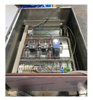
This picture shows the control panel box constructed to operate the ice machine. This was designed and built by M C Herd engineers. This box will be installed next to ice machine.
