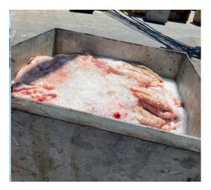
This photo depicts a full hide bin. As can be seen, once the bin has only just been pulled out from under the chute and place aside for truck loading and visually you can observe that the ice on top is not sufficient enough to cool the top hides. Random temperature checks taken have indicated hides in the middle and bottom of the bins are reaching target temperature of 10 degrees however hides on the top are not quite achieving this target.
