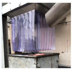
This photo shows the curtains which were installed around the bins to prevent the wind blowing the ice away when falling from the ice machine above. The hides are heavy enough that they fall through the curtains into the bin. As the ice is flaky is nature it didn't take long to notice that on days with even a slight breeze a large amount of ice was going to waste as it was blown onto the ground.
