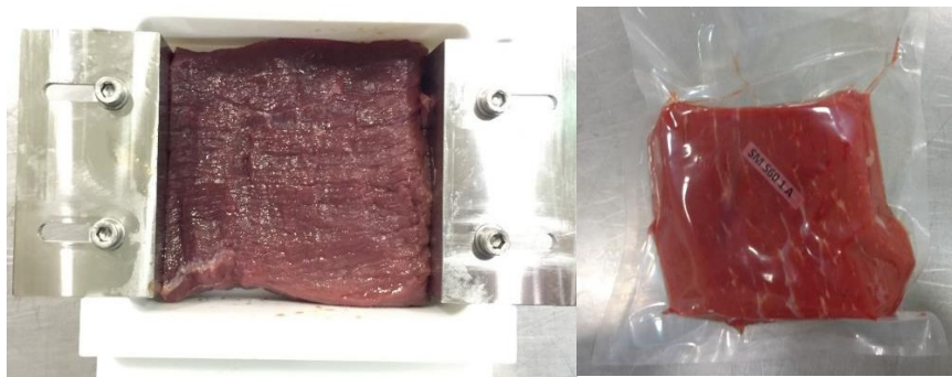
Figure 4-2. Left: Topside meat sample in a modified PEF treatment chamber for treatment of solid foods. Right: PEF treated topside meat sample vacuum packaged for ageing storage.
