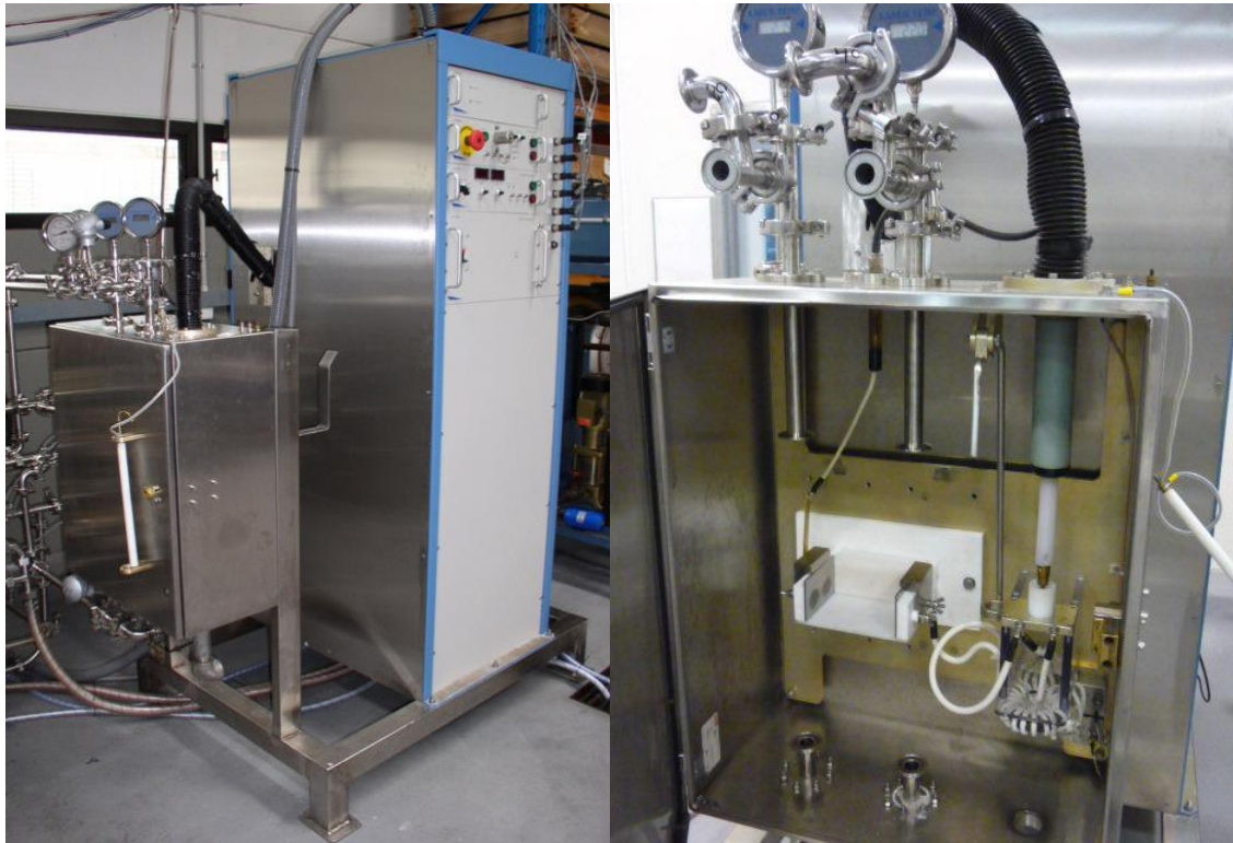
Figure 4-4. CSIRO's Power Mod™ 25 kW PEF System with PEF treatment chamber and modulator cabinet (left) and modified PEF treatment chamber set-up for processing of meat (right).
