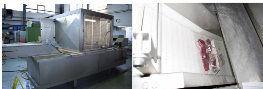
Figure 4-9. Left: The shockwave industrial prototype used in this experiment. Right: Meat samples being transported on the conveyor belt to the treatment area.
