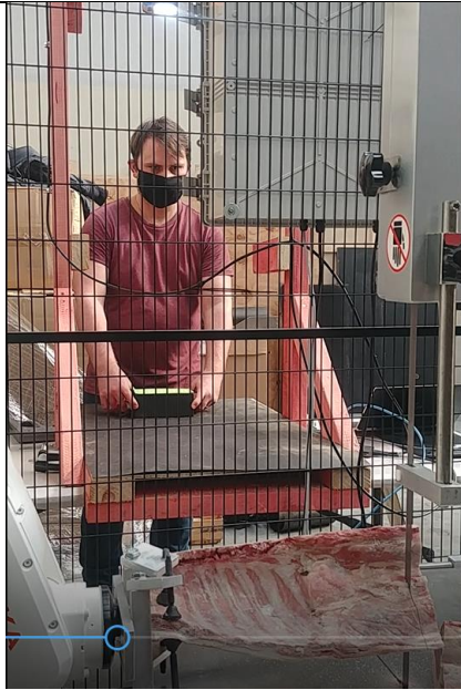
Figure 5 – Image of the system operating (extracted from a video) at an intermediate stage of development. The operator is lining up the cuts by 'eye', by watching the saw blade and adjusting the position of the meat by moving the 'box' in his hands.
