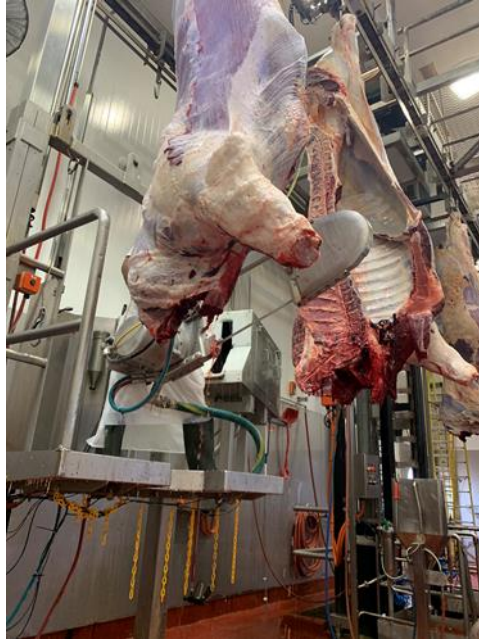
Figure 3: Splitting saw in operation showing build-up of bone dust and other material on the saw during operation.
