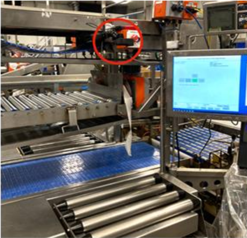
Fig 15: GoPro Data capture rig.
