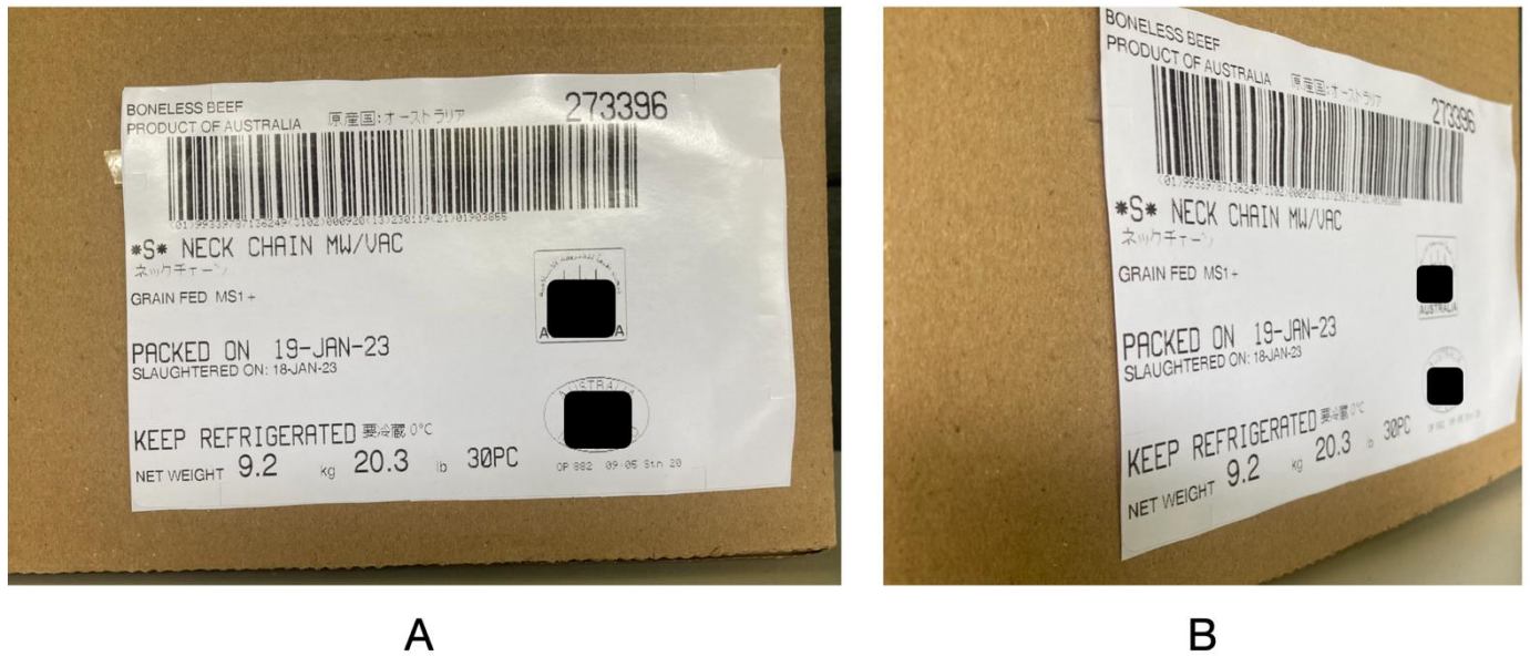
Fig 7. Impact of relative position of camera coordinate frame of reference to that of label on external surface of box of meat. Note the impact of defocussing of righthand side of image in B and the impact of lighting reflections in A.
