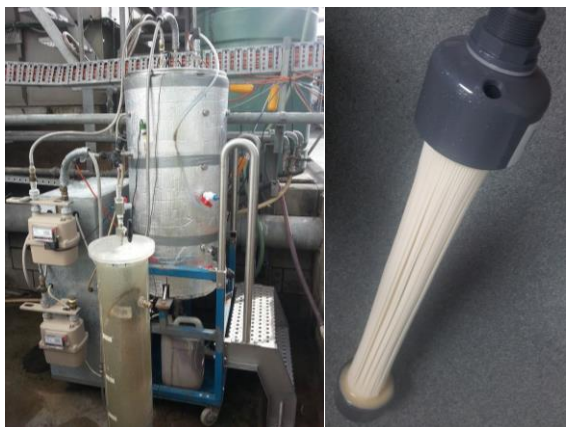
Figure 2: AnMBR Pilot Plant and hollow fibre membrane module.
