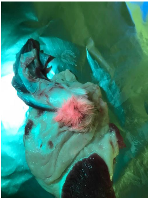
Figure 7. Left: Strong red fluorescence of wool samples under UV illumination (a UV filter was placed on the camera for this photo). Right: Same sample under normal illumination. The sample is from a mutton.
