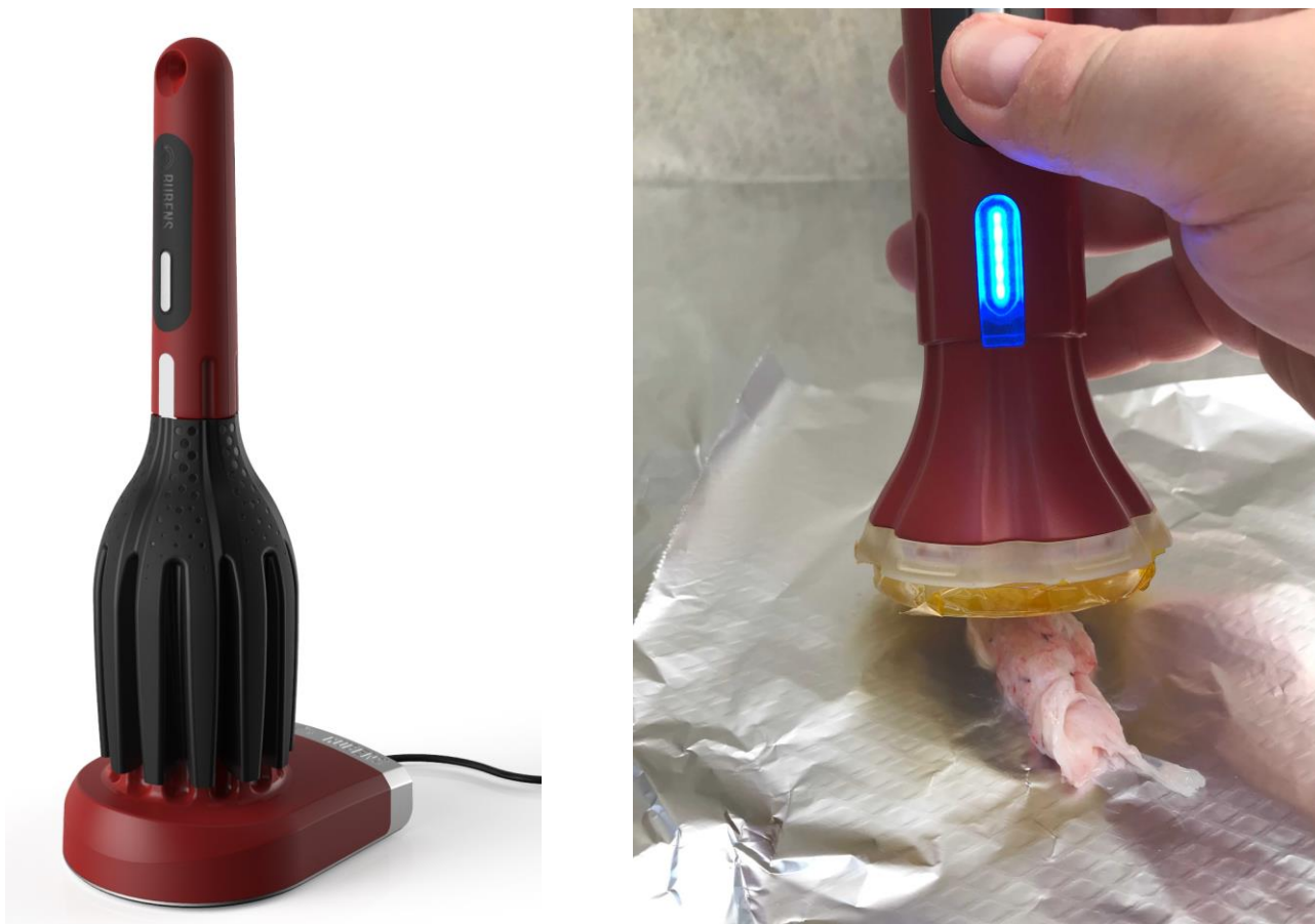
Figure 2. Left: Picture of the entire Rubens scanner, including the fruit shroud (dark grey) and its docking station. Right: Rubens scanning of a meat sample. The shroud was removed to allow for a close-up scan. Note that this photo was taken for the purpose of illustration only. The actual scans were taken in a dark environment, as explained in the text.
