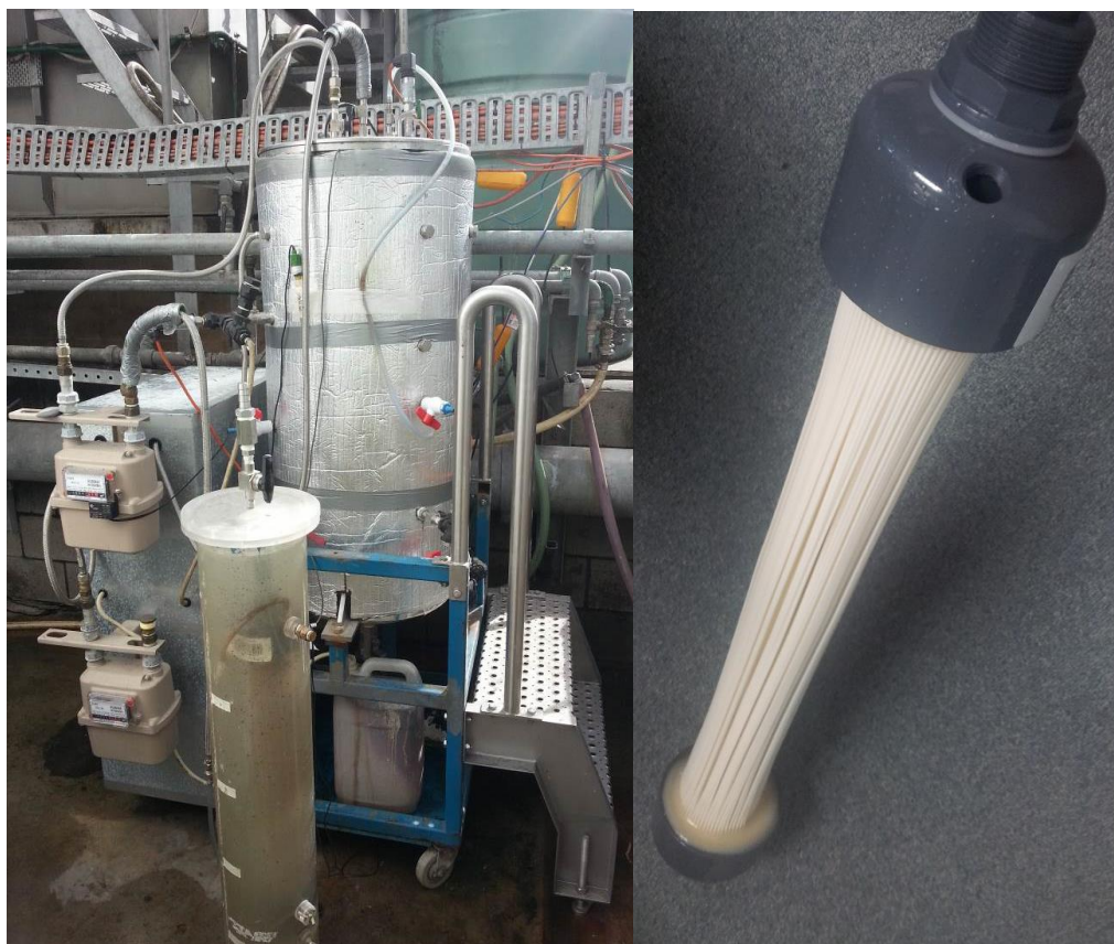
Figure 2: Anaerobic membrane bioreactor and hollow fibre membrane module
