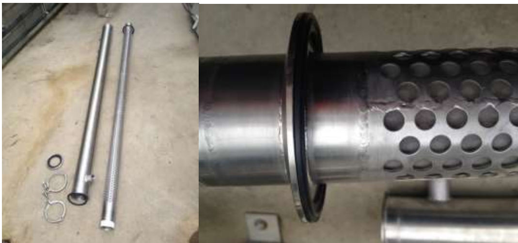
Figure 3: Custom-made stainless steel filtration module
