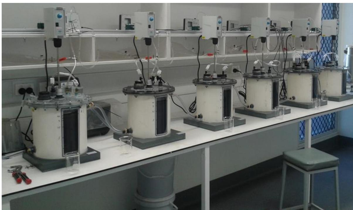
*Figure 6: Laboratory CSTR reactors used to determine the effect of temperature and agitation on crust/foaming layer development*
