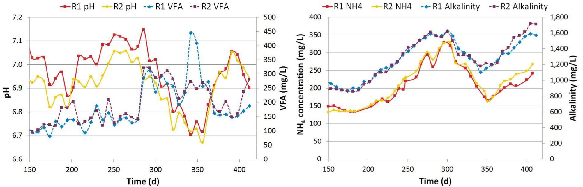
Figure 19: pH, VFA, NH<sub>4</sub> and alkalinity concentrations in the reactors
