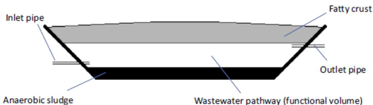
Figure 3: Illustration of dead space contributed by crust and sludge volume, resulting in a large reduction in functional pond volume, contributing to short circuiting (Harris & McCabe 2015).
