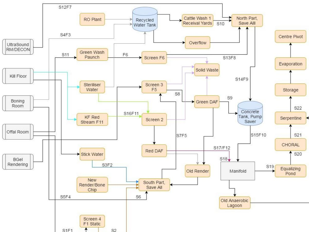
Figure 7: Detailed process schematic of waste water generation for Site A.
