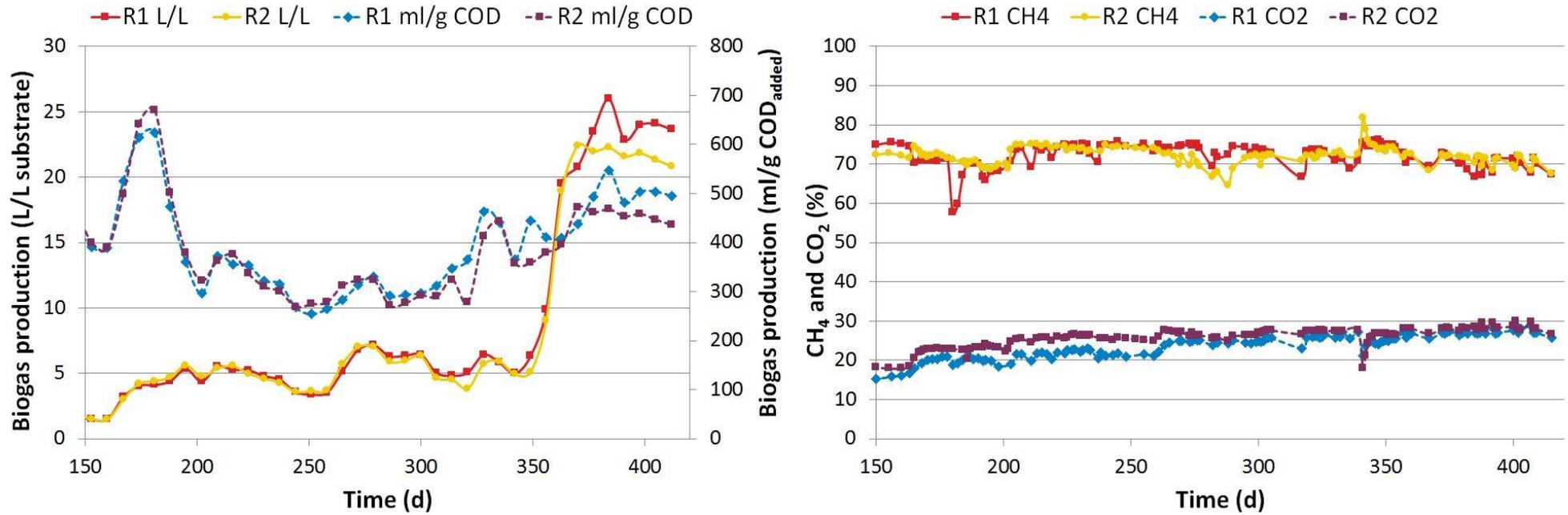
Figure 21: Biogas production per litre of feed stock and per g of COD added and concentrations of CH<sub>4</sub> and CO<sub>2</sub> in the biogas
