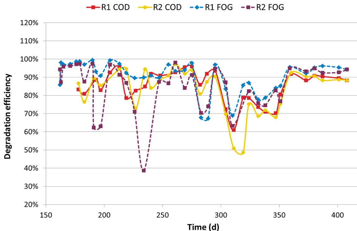
Figure 20: COD and FOG degradation efficiency in the reactors
