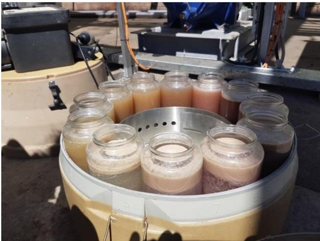
Figure 10: Autosampler collection at combined saveall waste flow (S15) showing clear variability amongst samples over a 24 hour period.
