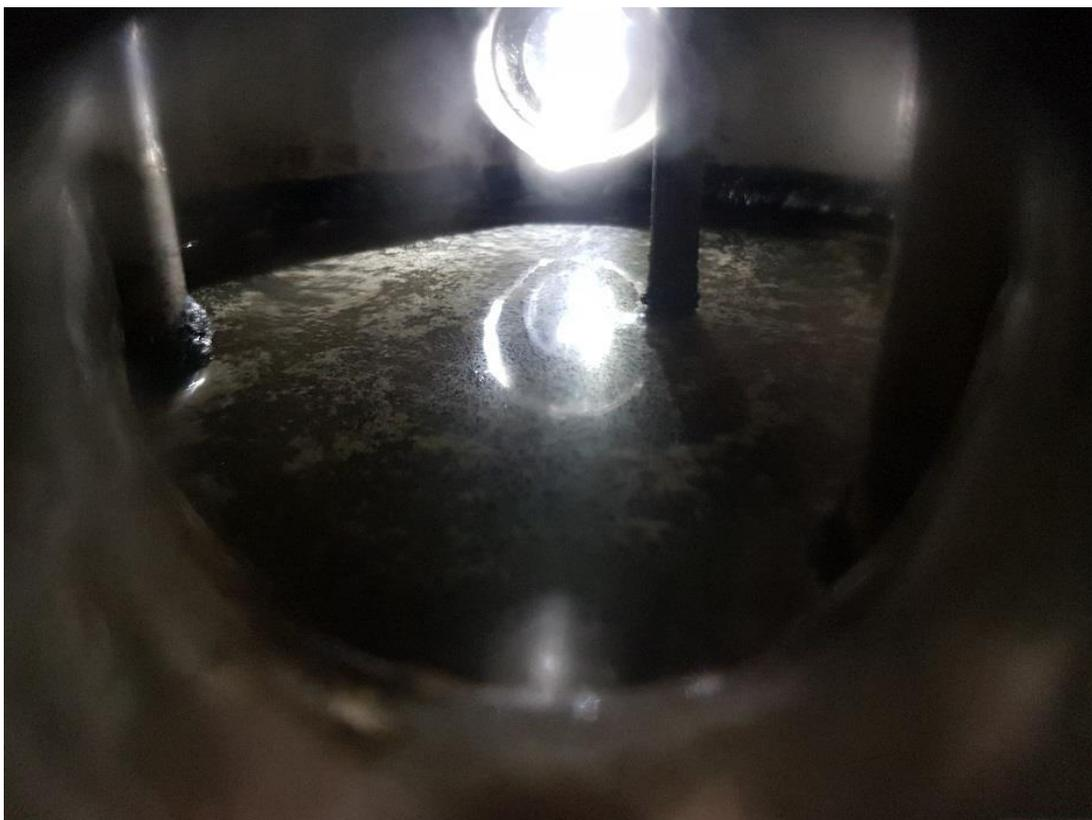
*Figure 18: View of surface layer in lab scale reactor showing no evidence of scum/foaming*
