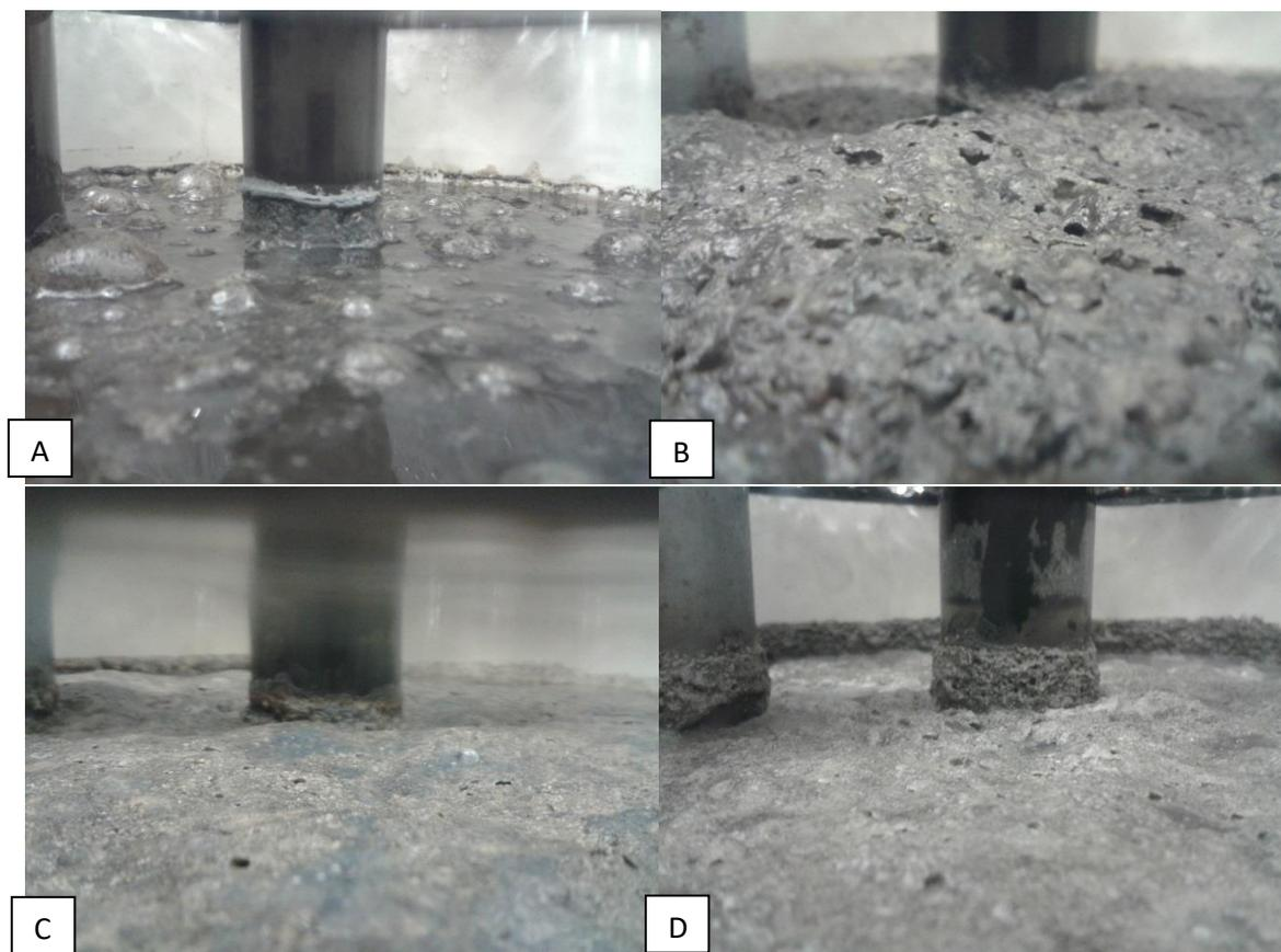
Figure 22: Crust/foaming layer in the reactors with minimal stirring on day 4 (A), day 16 (B), day 43 (C), and day 57 (D)
