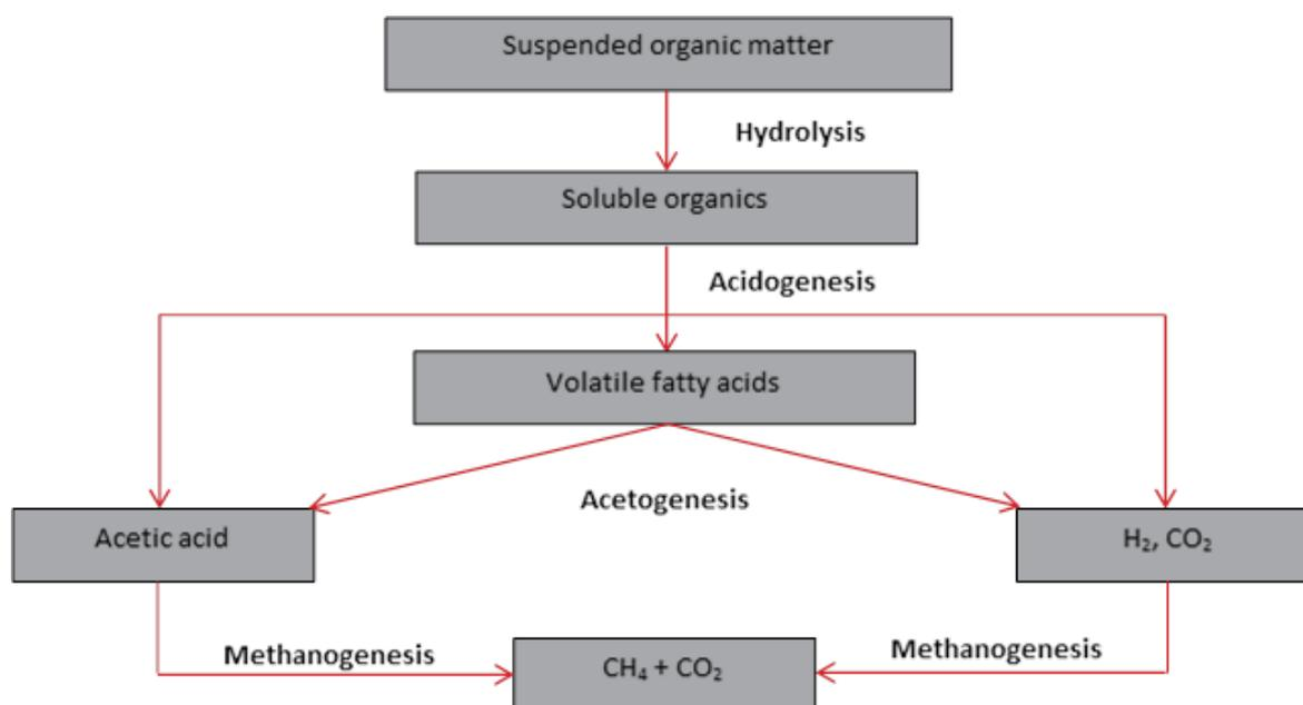
Figure 2: Stages of anaerobic digestion, modified from (Appels *et al.* 2008)
