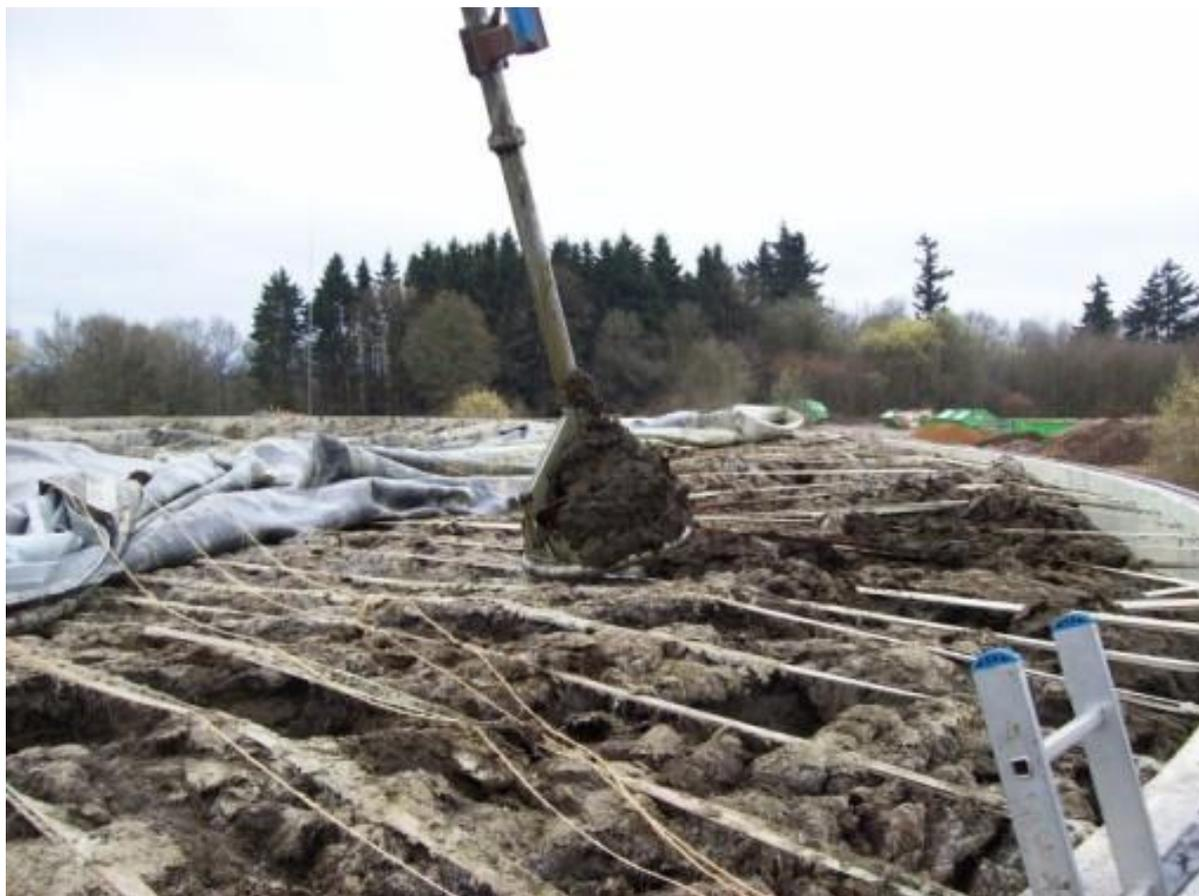
*Figure 1: Floating layer in an agricultural biogas plant in Germany after failure of agitator (Feuerborn 2016)*
