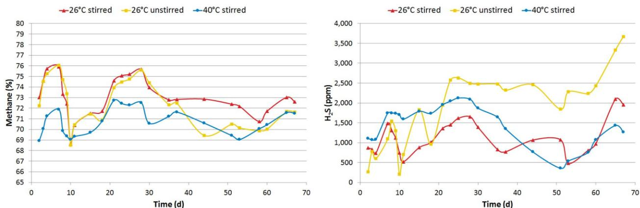
Figure 27: Methane and H<sub>2</sub>S content in the reactors
