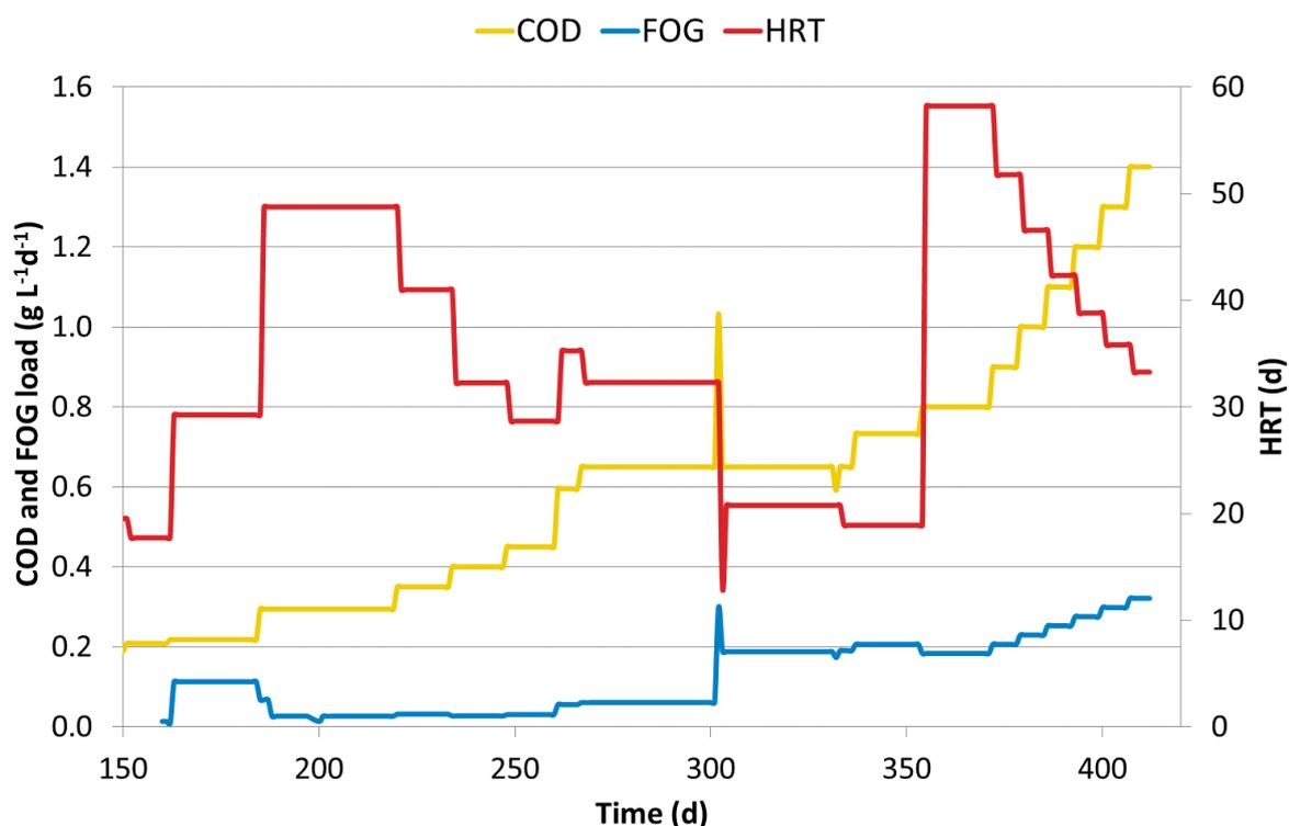
Figure 17: COD and FOG load; HRT in the reactors
