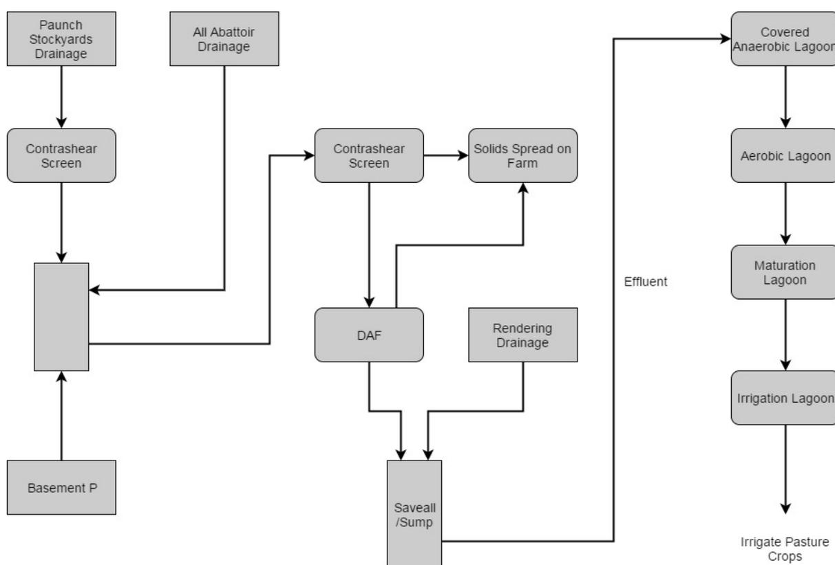
Figure 9: Effluent flow schematic at Site C.
