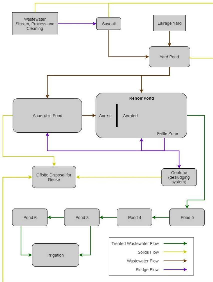
Figure 8: Waste water treatment flow chart for Site B
