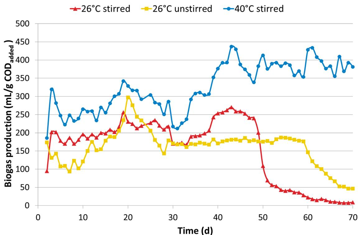
Figure 26: Biogas production in mL/g COD<sub>added</sub> in the reactors
