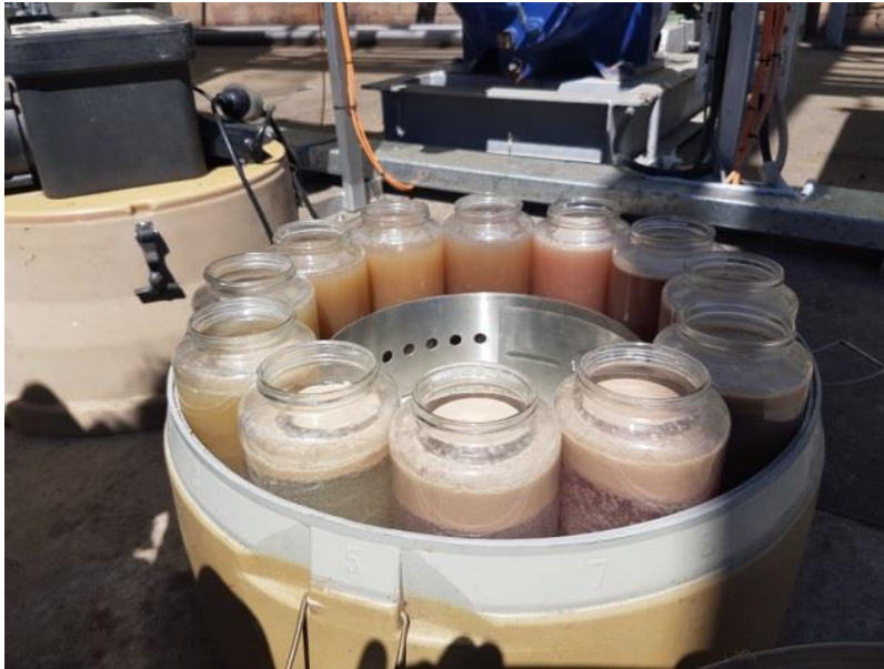
Figure 4: Autosampler collection at combined saveall waste flow showing clear variability amongst samples collected over a 24 hour period.
