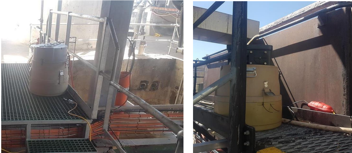
Figure 3: ISCO autosampler on saveall south waste stream (S6) (left) and saveall south post-screen waste stream (S8) (right).
