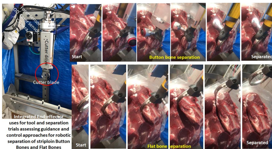
Figure 11: Cutter end-effector separation trial with button and flat bones.
