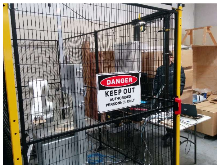
Figure 1 – Photo of the set-up including the safety fencing within which sits the robot and bandsaw.
