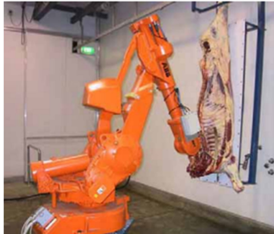
Figure 15 Robot scribing station prototype (Starling, 2003)
