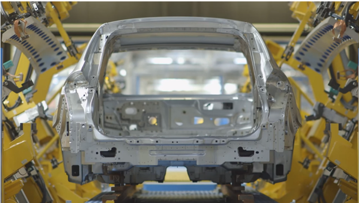
Figure 21 Panels are welded together to form the assemblies, then Bodyshell, and finally Body In White (Europe, 2015)
