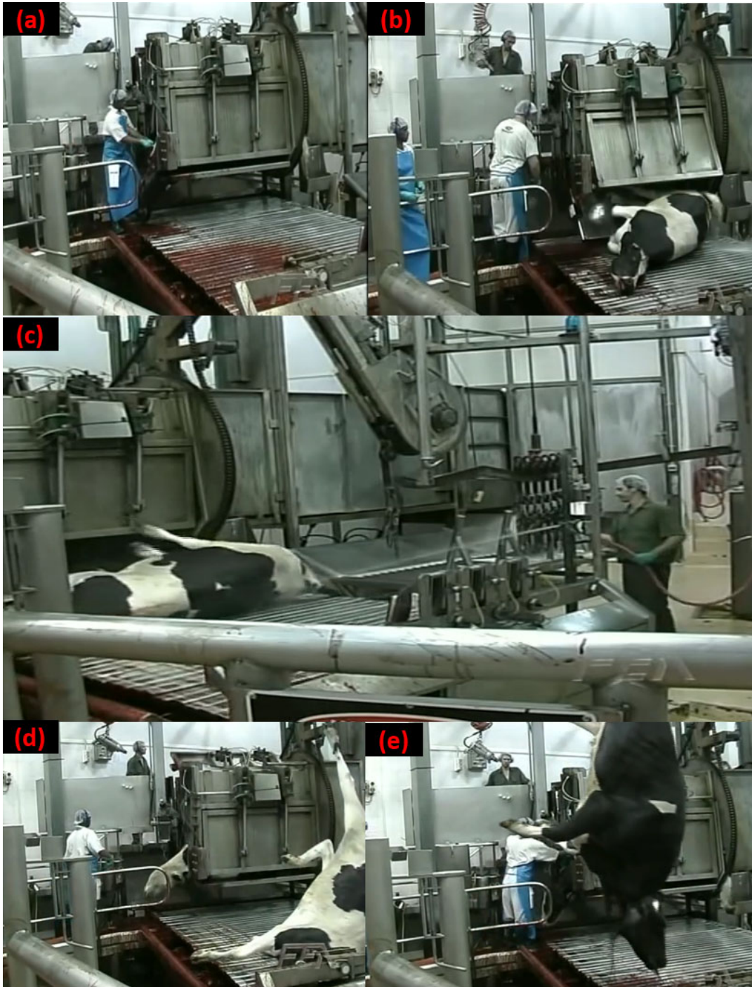
Figure 11 Sticking, post stunning wash and hanging. (a) Immediately after stunning happens the severance of the carotid artery and jugular vein takes place in a horizontal position “sticking”. (b, c) The carcass is lowered onto a moving stainless-steel rail where post stunning wash takes place. (d, e) Suspension by the hind leg and held in a vertical position for maximal blood removal (Foodequip, 2009)
