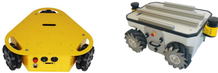
Figure 9.3.3 AGVs with Omnidirectional wheels and Mecanum wheels
