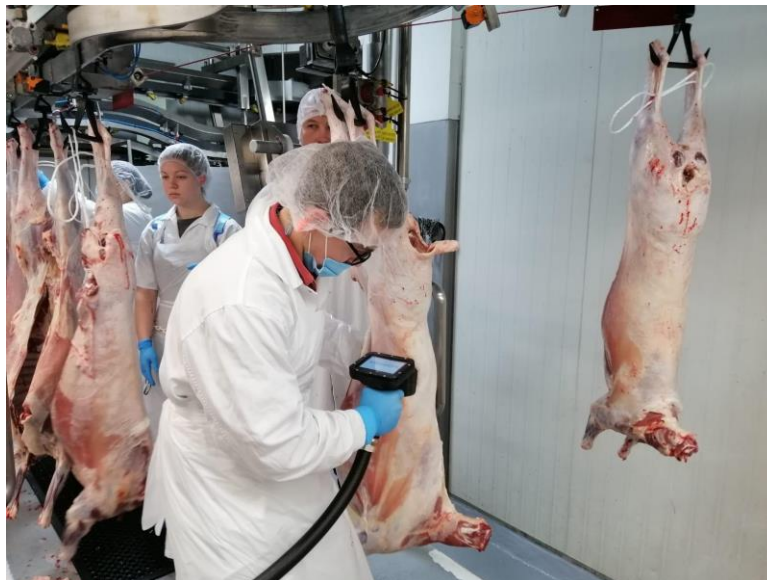
Figure 1: Callan Daley (MEQ Field Team Member) probing carcasses with the MEQ Probe
