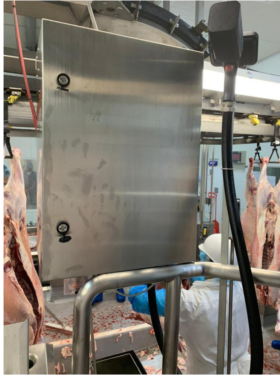
Figure 2: Photo of MEQ unit that powers the probe and the probe in its holster.
