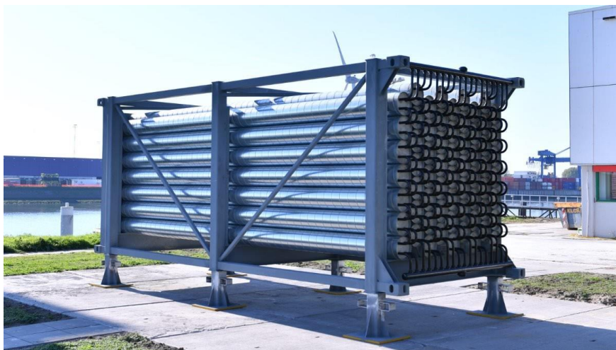
Figure 48. Modular TES technology from Energy-Nest [173].
