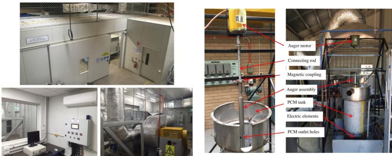
Figure 55. Left: High-temperature test facility; Right: auger melting rig at the University of South Australia [195].
