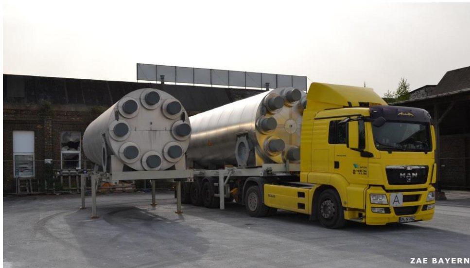
Figure 46. Mobile TES from waste heat source [158].
