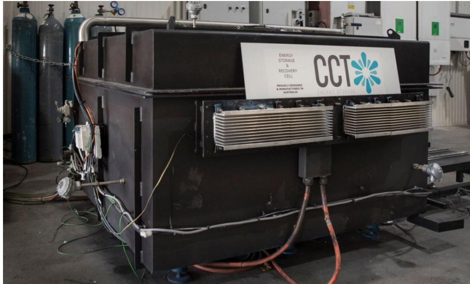
Figure 52. CCT Energy Storage's thermal battery [188].
