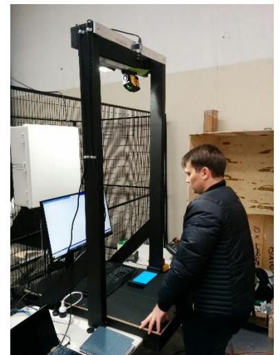
Figure 1 – Photo's of the set-up including the safety fencing within which sits the robot and bandsaw and outside the cage, the object tracking table (right).
