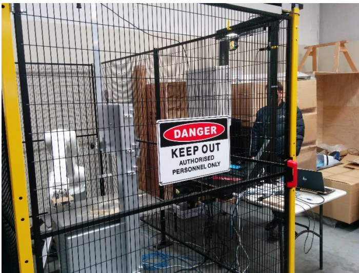
Figure 1 – Photo's of the set-up including the safety fencing within which sits the robot and bandsaw and outside the cage, the object tracking table (right).
