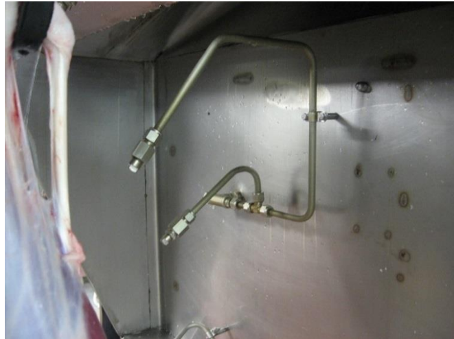
Image 3: Sprays deliver hot water between 60-65°C at the surface of the carcass for three seconds at 16 bar pressure.
