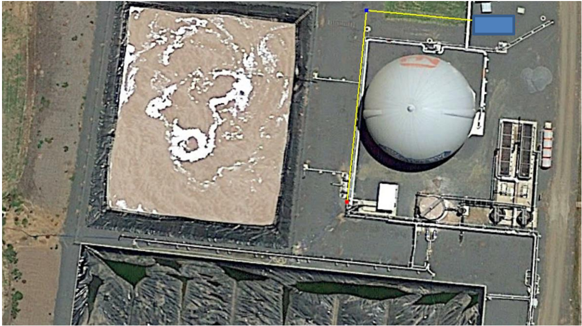
Figure 2: Assumed engine location (blue rectangle) and thermal fluid reticulation (yellow line) for heating liquid existing feed pond (upper left) and entering the main COHRAL system (at bottom of image).
