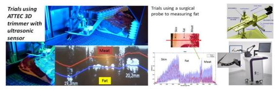
Fat on beef striploins can, in some sections, be delaminate or have air gaps (bubbles) within their structure. The sensing approach measuring fat-lean profile from the lean side, as well as trimming the fat under cross sectional pressure minimizes or avoids complications related to delamination or air bubbles.
