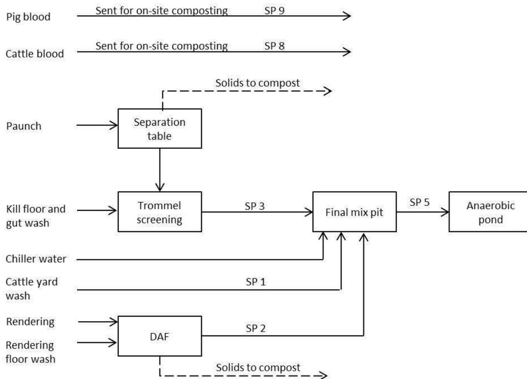
**Figure A1.6. Flowsheet of wastewater sources, handling and treatment at Site F (adapted from Jensen and Batstone, 2012). SP: sample point.**
