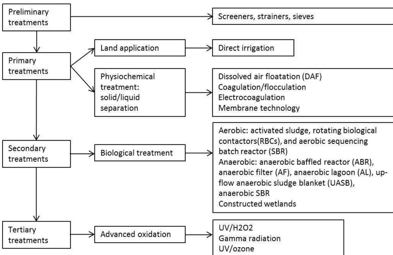
**Figure 4. Abattoir wastewater treatment process.**
