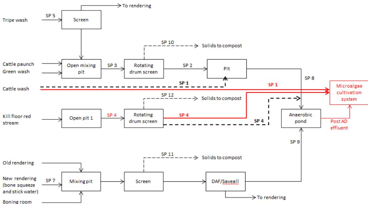
**Figure A3.3. Reconfiguration of the process flowsheet at Site A. Black dotted lines: current flowsheet. Red lines: proposed reconfiguration by directing streams SP1 and SP4 to microalgae cultivation. SP: sample point.**
