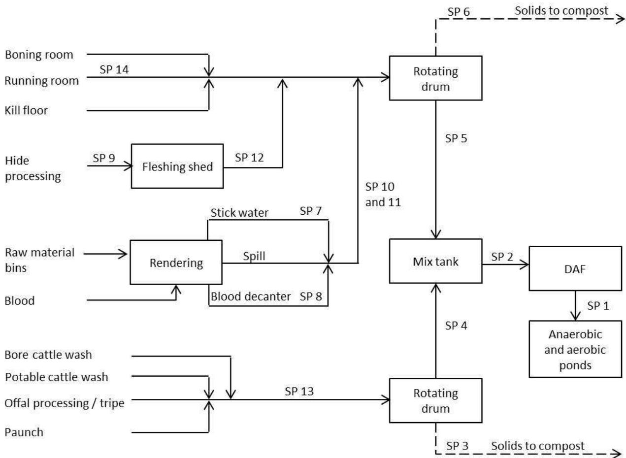
**Figure A1.5. Flowsheet of wastewater sources, handling and treatment at Site E (adapted from Jensen and Batstone, 2013). SP: sample point.**
