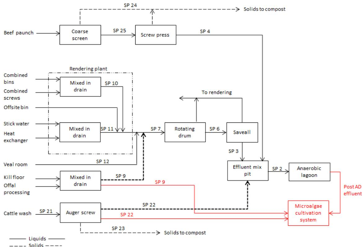
**Figure A3.4. Reconfiguration of the process flowsheet at Site D. Black dotted lines: current flowsheet. Red lines: proposed reconfiguration by directing streams SP9 and SP22 to microalgae cultivation. SP: sample point.**
