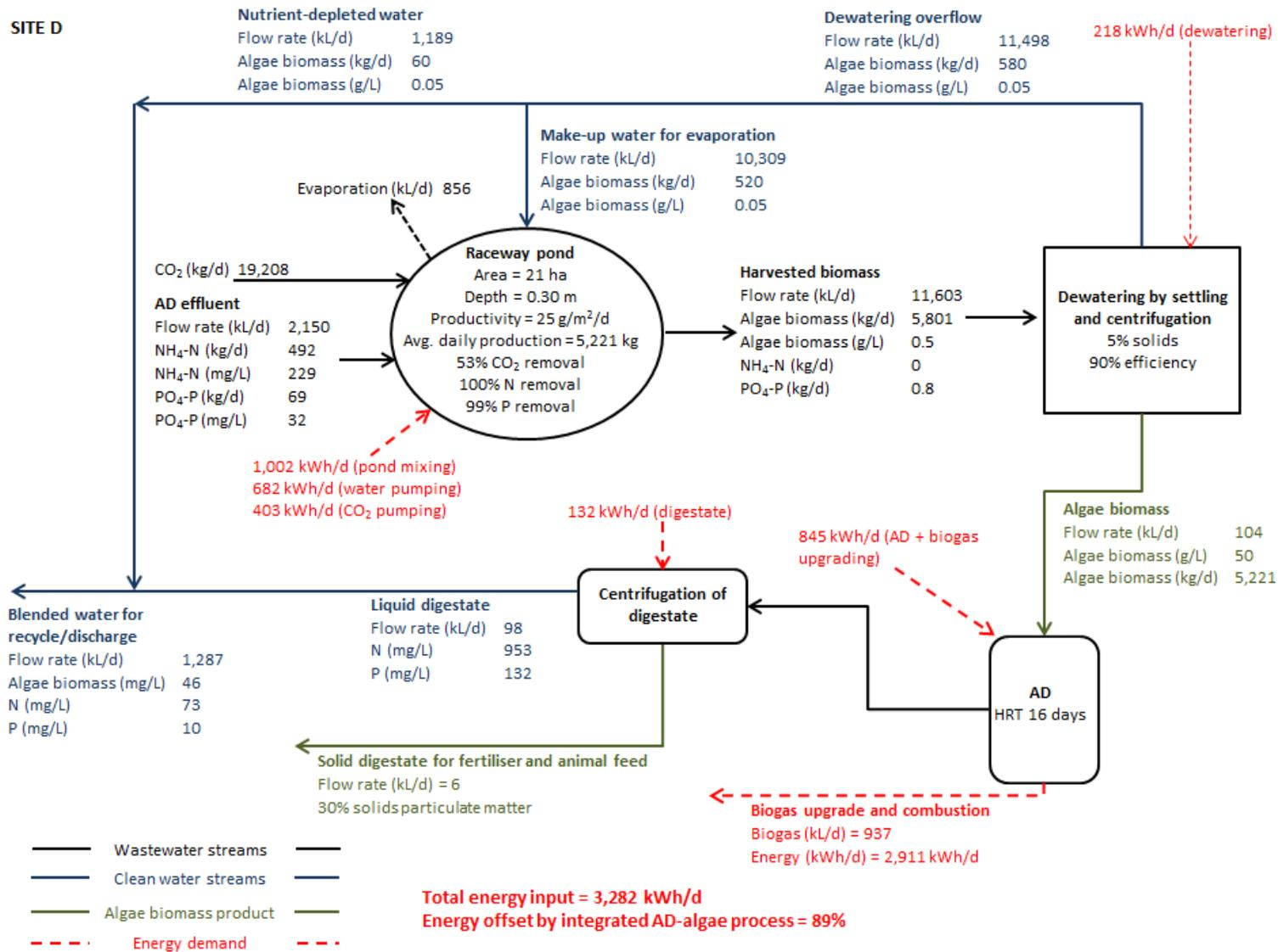
Figure 8. Mass and energy balances of the integrated AD - microalgae cultivation system at Site D.
