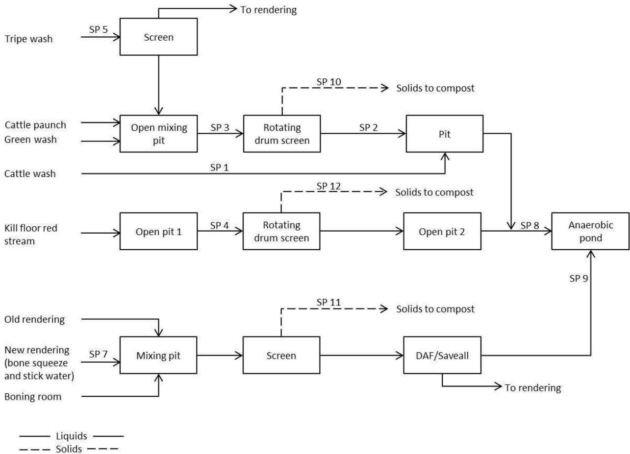
**Figure A1.1. Flowsheet of wastewater sources, handling and treatment at Site A (adapted from Jensen and Batstone, 2012). SP: sample point.**
