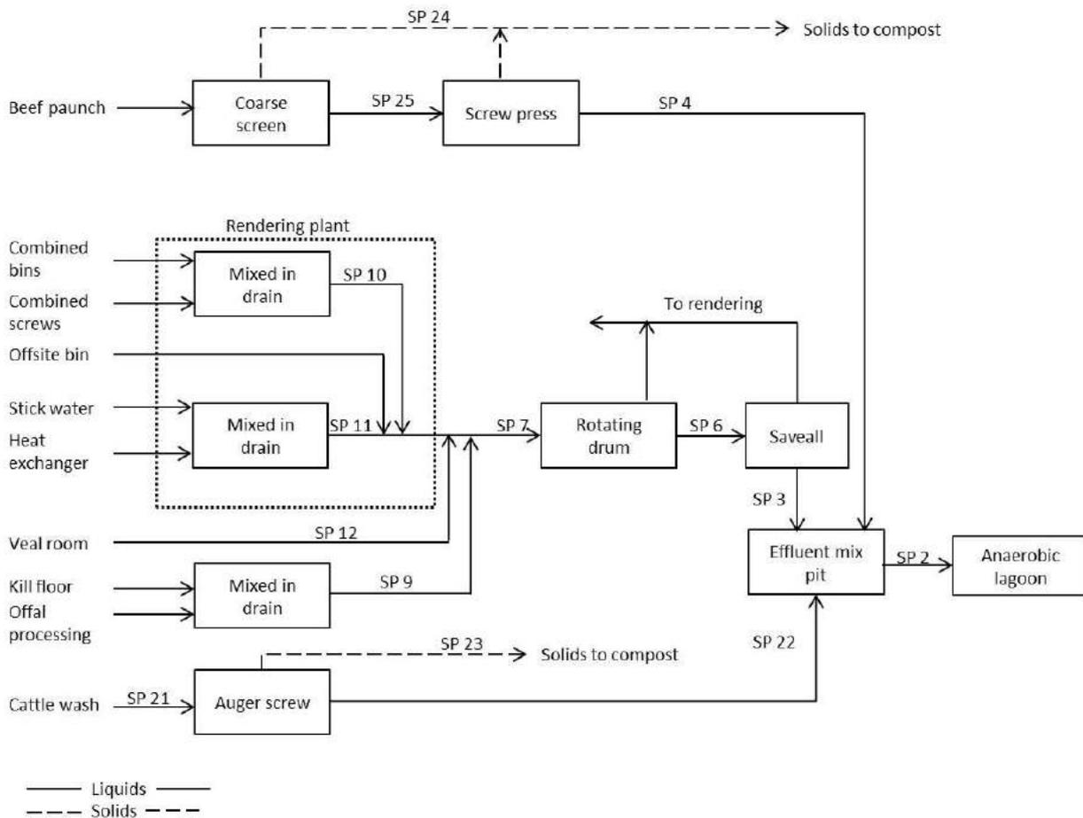
**Figure A1.4. Flowsheet of wastewater sources, handling and treatment at Site D (adapted from Jensen and Batstone, 2013). SP: sample point.**
