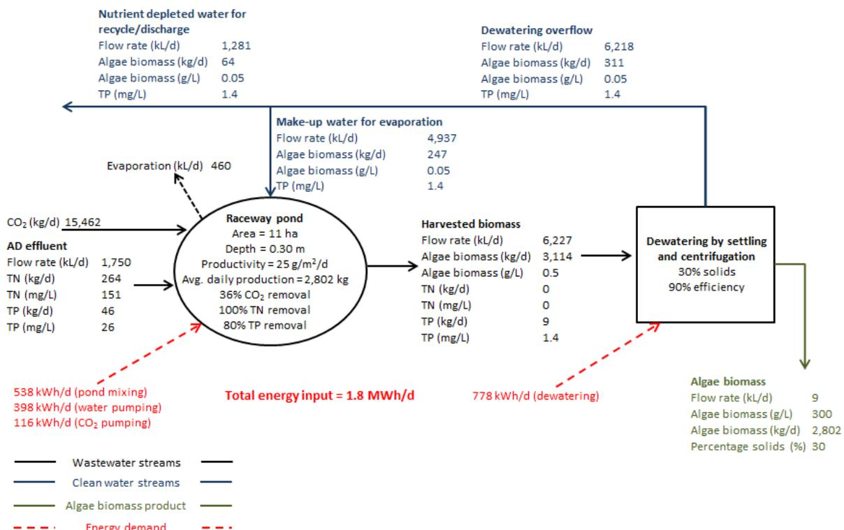
**Figure 6. Mass balance and system sizing of the microalgae cultivation system at Site G. Wastewater stream sent to microalgae cultivation: AD effluent.**
