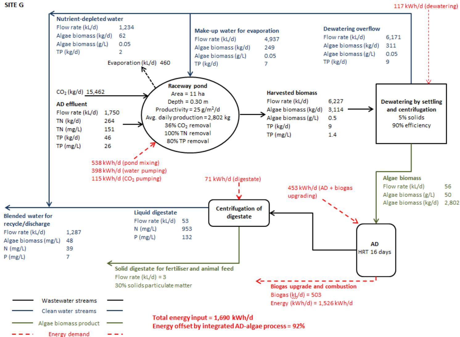
Figure 9. Mass and energy balances of the integrated AD - microalgae cultivation system at Site G.
