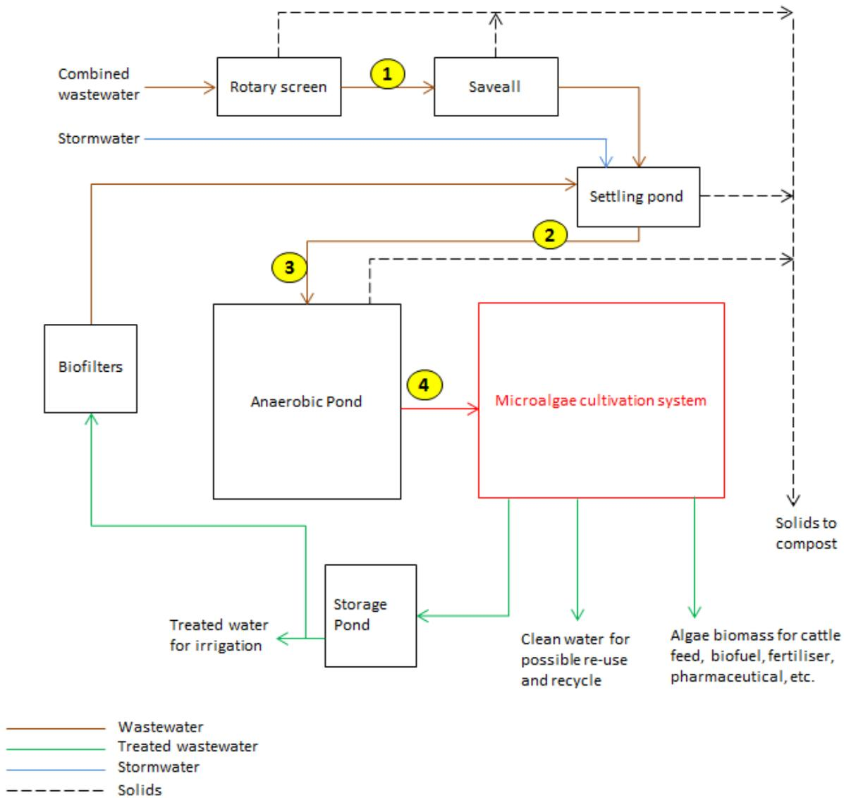
**Figure A3.1. Flowsheet of the wastewater treatment plant at Site G which includes the proposed microalgae cultivation process (highlighted in red) applied on the AD effluent (Stream 4).**
