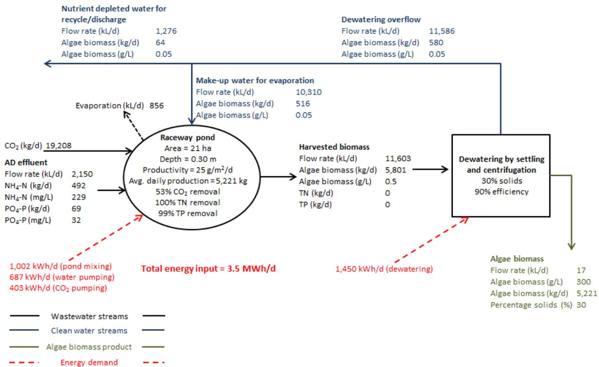
**Figure 5. Mass balance and system sizing of the microalgae cultivation system at Site D. Wastewater stream sent to microalgae cultivation: AD effluent.**
