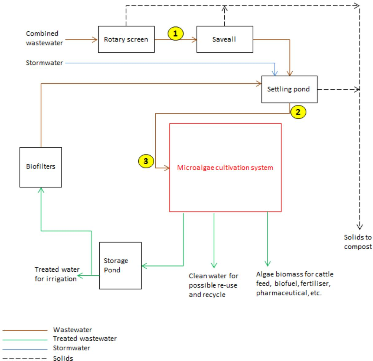
**Figure A3.2. Flowsheet of the wastewater treatment plant at Site G which includes the proposed microalgae cultivation process (highlighted in red) applied on the primarily treated wastewater effluent (Stream 3).**
