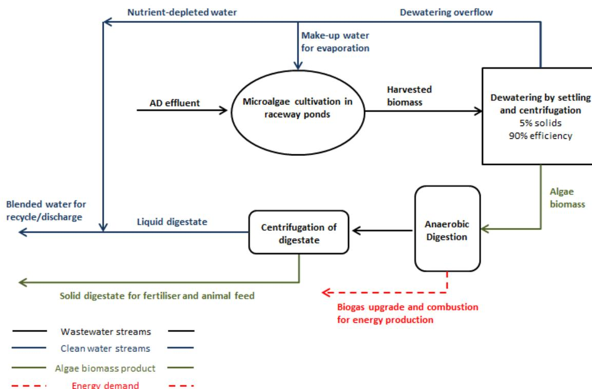
Figure 7. Schematic process flowsheet diagram of the integrated AD-microalgae cultivation system.
