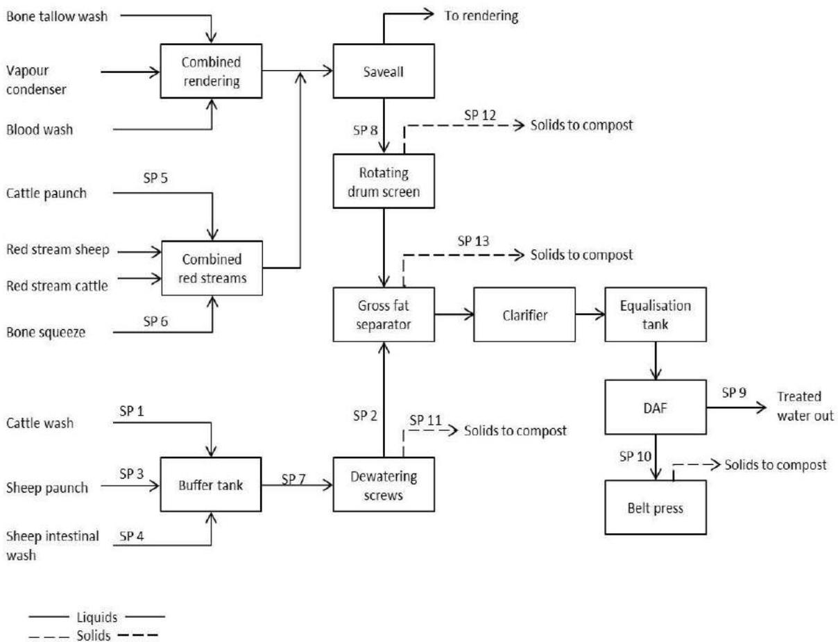
**Figure A1.2. Flowsheet of wastewater sources, handling and treatment at Site B (adapted from Jensen and Batstone, 2012). SP: sample point.**
