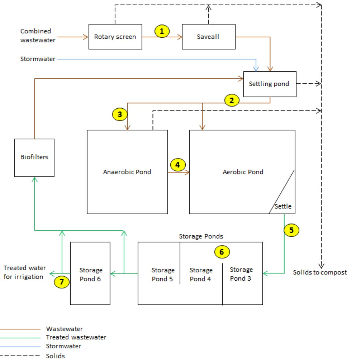
**Figure A1.7. Flowsheet of the wastewater treatment plant at Site G. Water quality sampling points are highlighted.**
