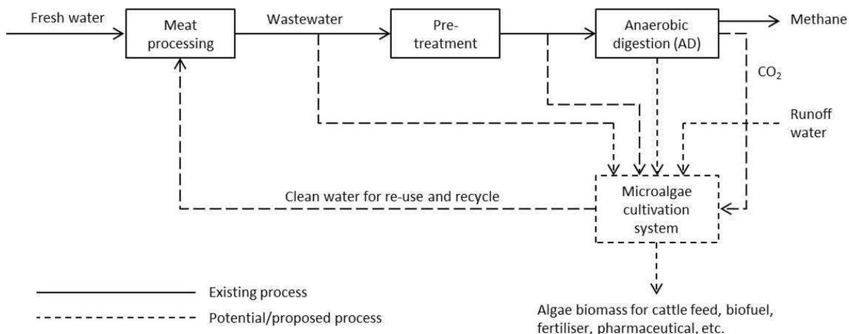
**Figure 1. Integration of microalgae cultivation with the wastewater treatment process.**
