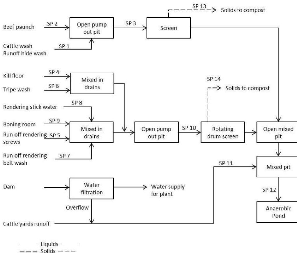
**Figure A1.3. Flowsheet of wastewater sources, handling and treatment at Site C (adapted from Jensen and Batstone, 2012). SP: sample point.**
