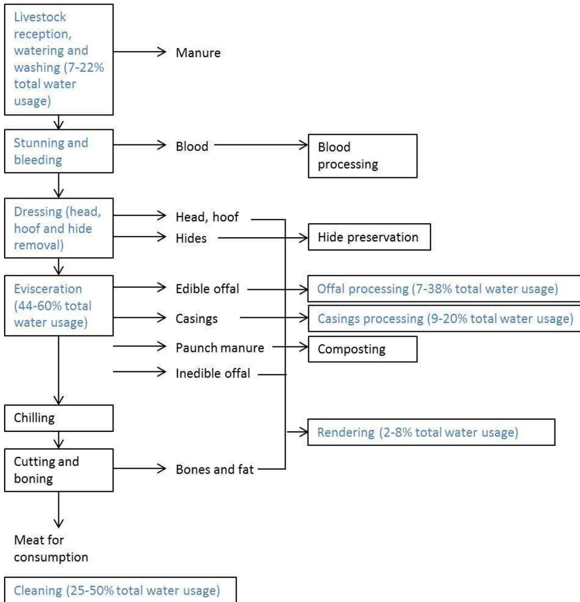
**Figure 3. Process flow diagram of red meat processing operations. Operations with a substantial water consumption rate are highlighted in blue (COWI, 2000).**
