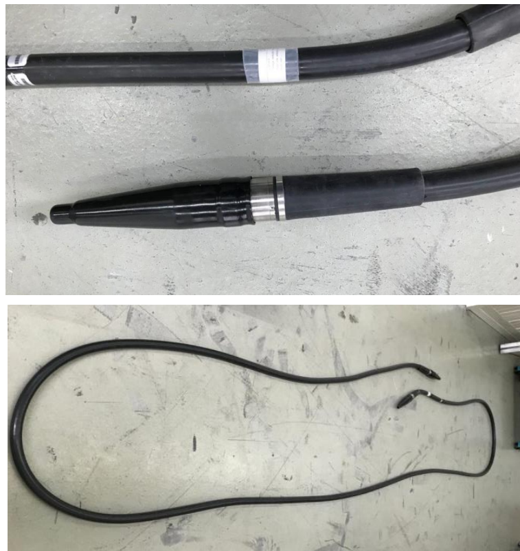
Figure 2: Cable Condition - Post Cycle Testing
