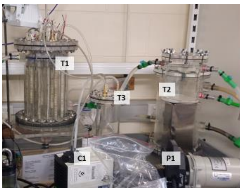
Figure 9: Attached growth schematic setup and laboratory configuration. (T1) photo-bioreactor; (T2) sampling reservoir; (T3) water trap (avoiding moist return towards the air compressor); (C1) air compressor for gas phase recirculation (from headspace to the bottom of the reactor); (P1) Feed pump.
