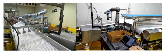
The Vision System successfully identified the selected primal cuts by size and volume to complete the Trial at Scone. For future installations additional AI and Deep learning technology will also be implemented with the Vision System to create a very robust final solution for this application.
