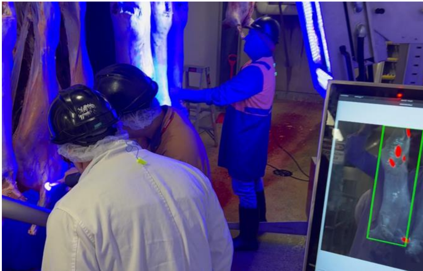
Figure 1: Localised BluLine Spot detection (bottom left). BluMax carcass detection (centre and right)
