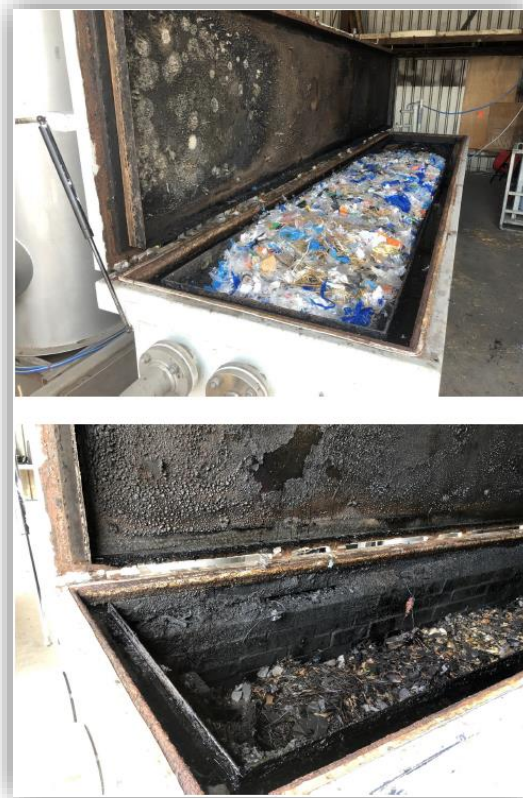
Figure 1: Gasification reactor showing mulched mix of paper, cardboard, and plastic, and residual char
