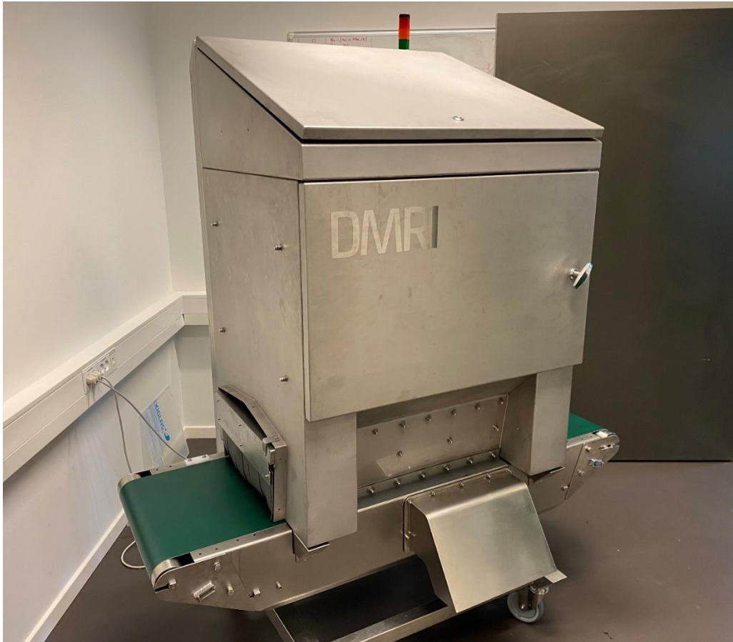
Figure 1. The test unit combining vision and x-ray technology mounted with a moving conveyor with a green belt.
