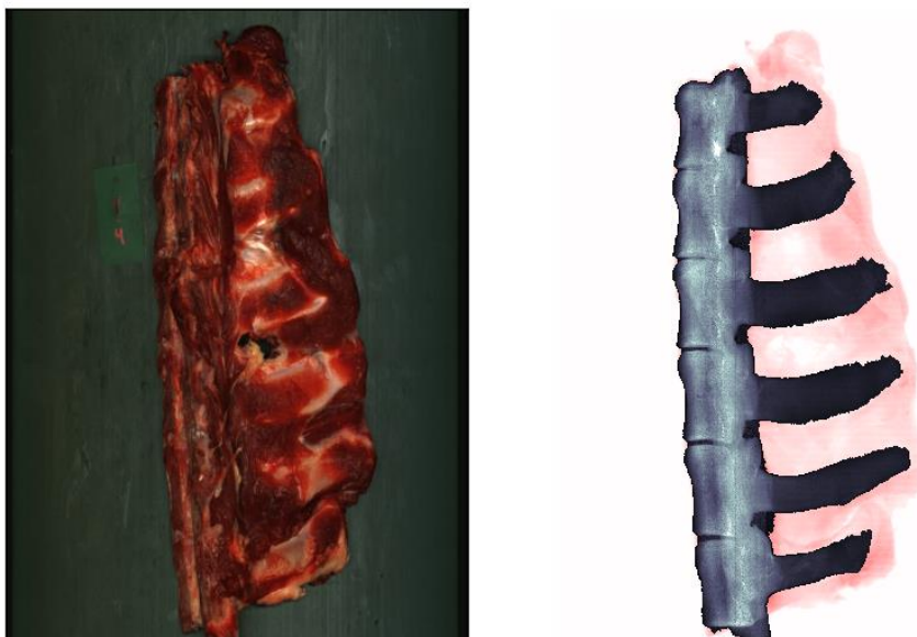
Figure 7. Meat and bone segmentation for a loin bone using DEXA data. The estimated meat-to-product ratio (here 32.5%) is volume-based. Cartilage at the bone edges is grouped with meat.
