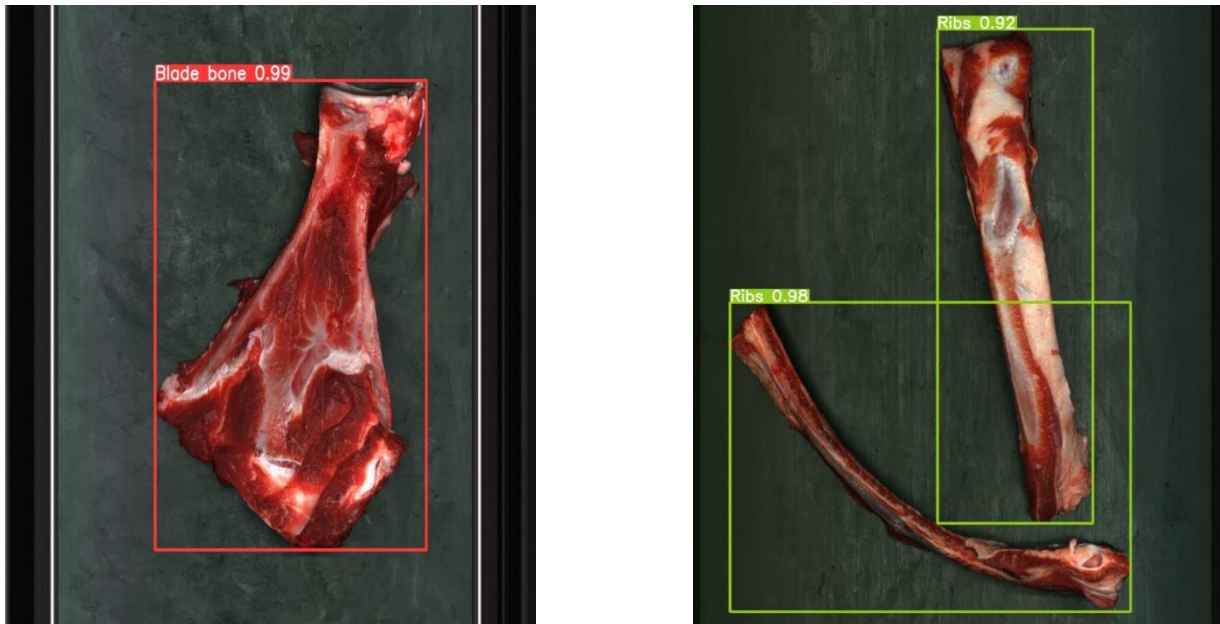
Figure 6. Example of two different types of bone segments located with a bounding box and identified with a score of certainty (from 0-1). The left bone segment is recognized as a blade bone (Scapula) and to the right, two ribs are identified and located correctly as well.
