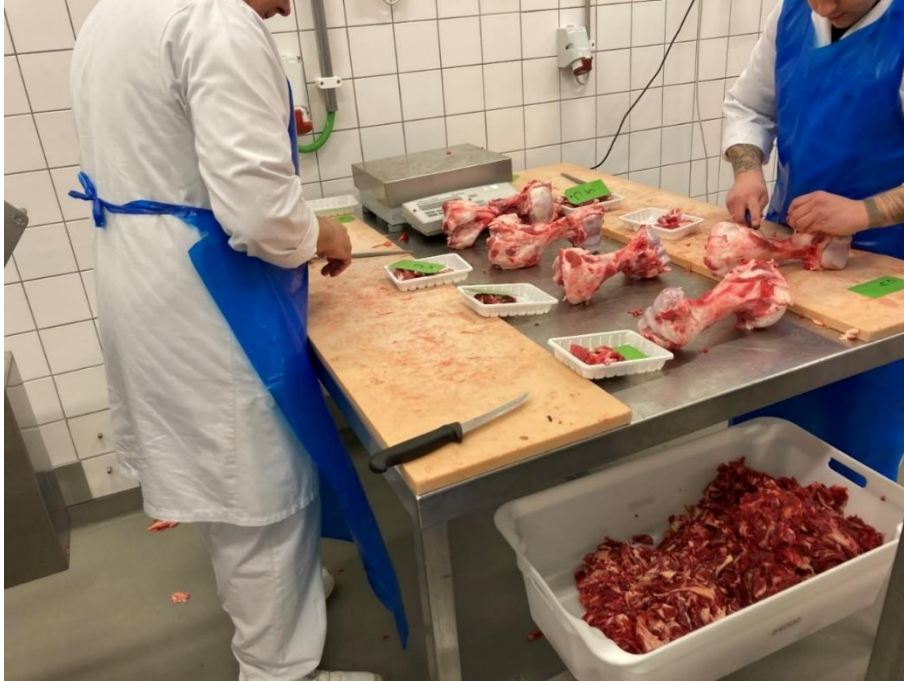
Figure 4. Trimming operators working on different bones in steps to ensure corresponding data consisting of measurement scans and the registration of weight of recoverable meat for each of the five trim scores.
