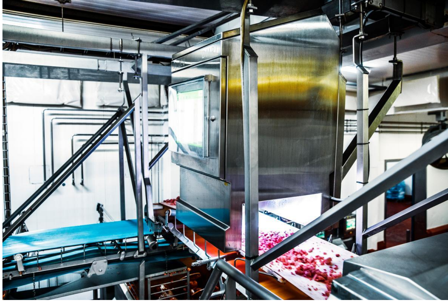
Figure 1. A Vision unit mounted above a conveyor line in a meat processing facility.
