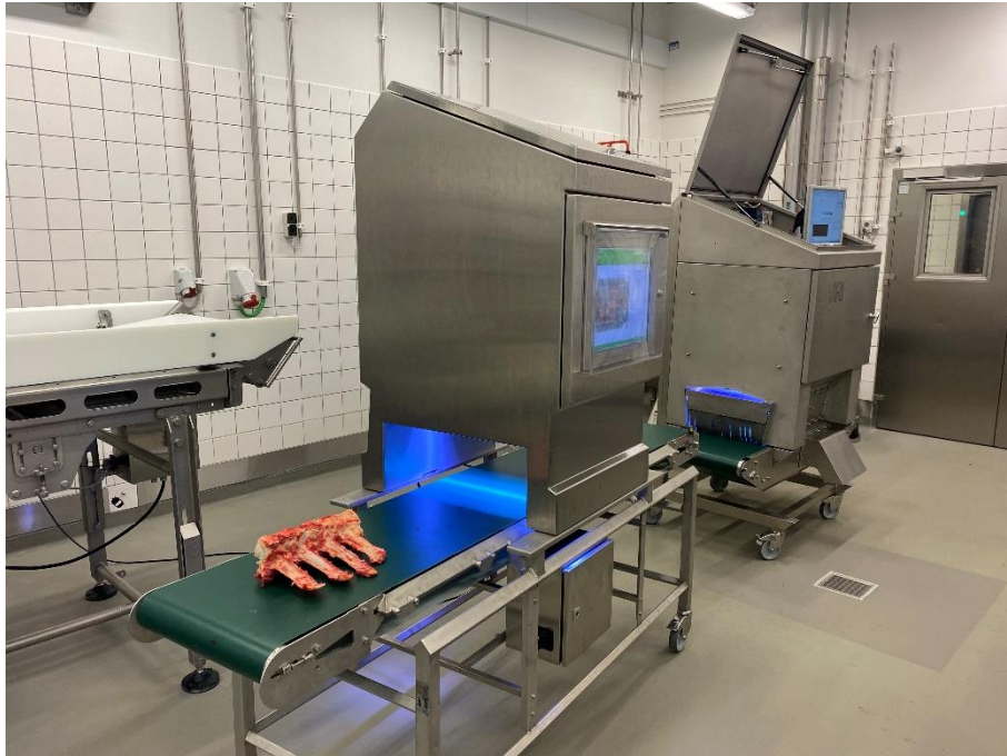
Figure 2. Example of the scanning of a single loin bone (Lumbar Vertebrae) using the adapted Vision Measurement System (seen in front).
