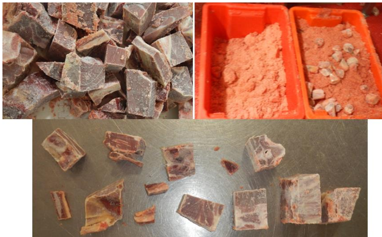
Figure 24: Band-saw bone dust and variability in cube size.
