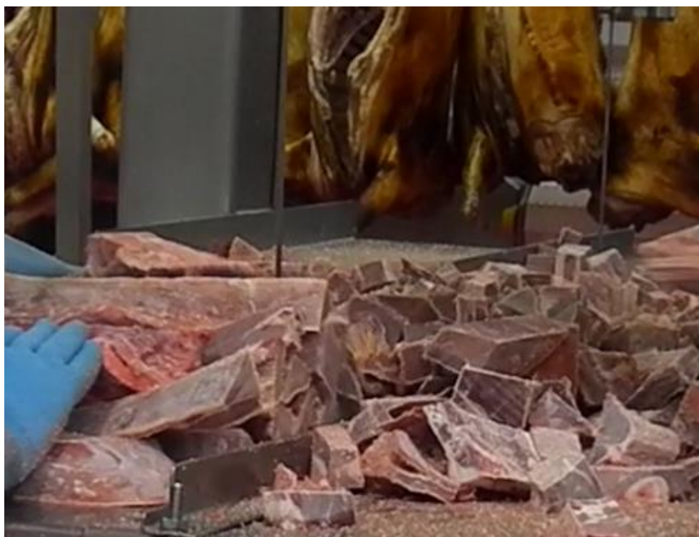
Figure 22: Typical set up cutting cubes on a band-saw (confidential).
