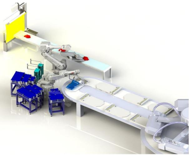
Figure 22: Concept design for a completely automated primal cut bagging system, of which the naked primal cut recognition vision system is an integral component. (Source: AMPC Project No: 2018-1049 Automation of Primal Cut Bagging)
