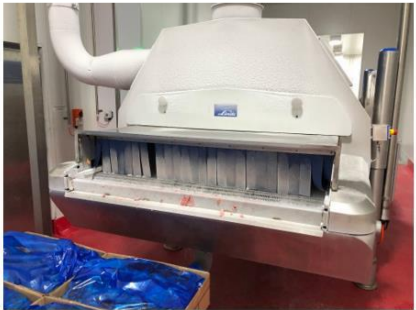
Fig 4 cooling tunnel in operation test phase
