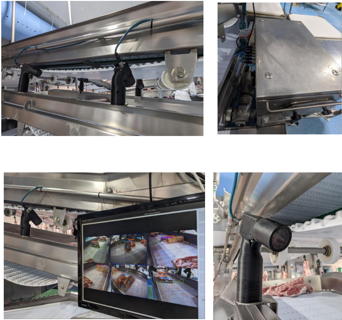
Figure 10: Components of the advanced hardware design. Clockwise from top left: Cameras mounted in place, computer system housing, camera on fixed angle mount, screen for real-time tracking.
