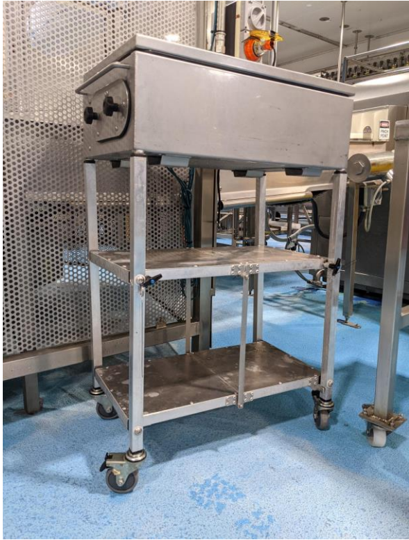
Figure 2: Stainless steel computer housing and trolley for easy relocation.
