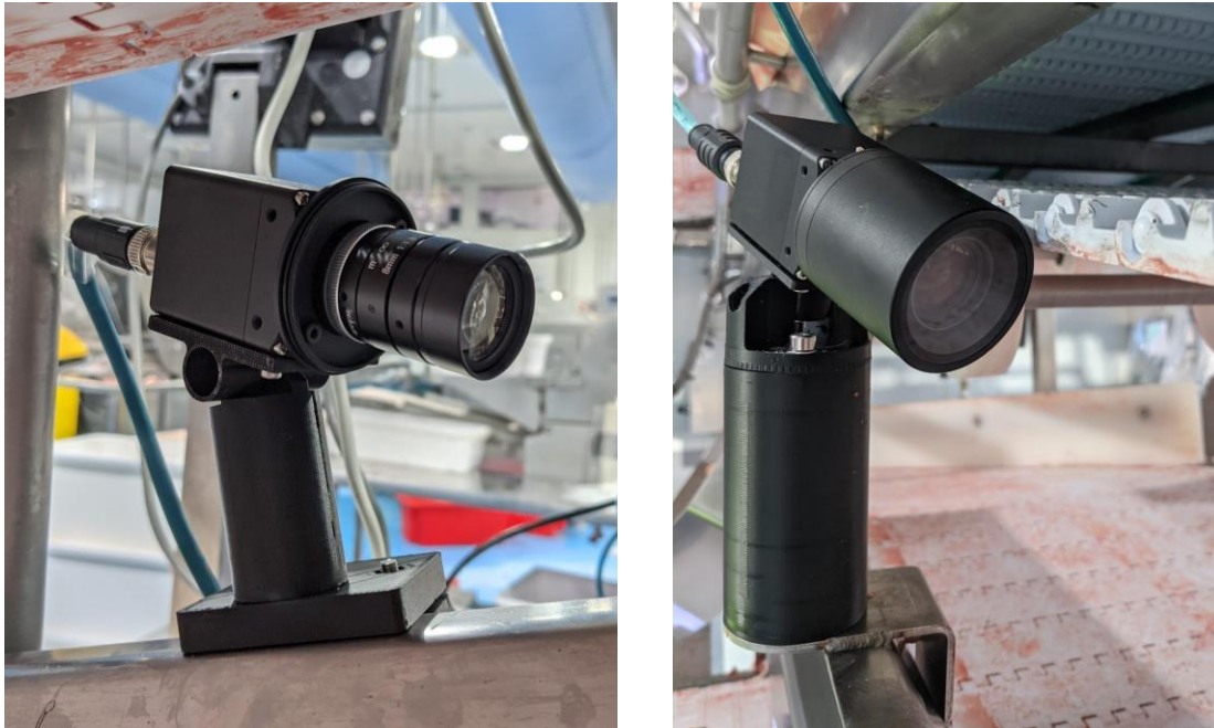
Figure 4: Version one camera mounting system (left); Version two camera mounting system with fixed position (right)
