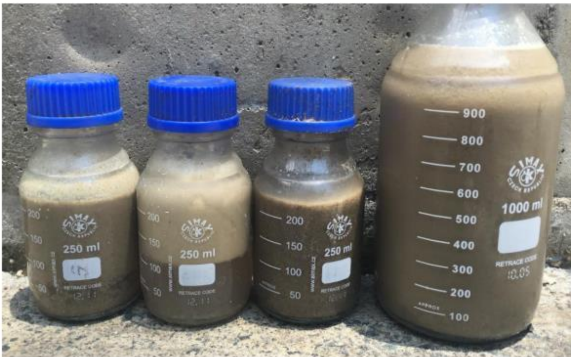
Figure 9: DAF float hydrocyclone visual results shows, from left: DAF float inlet, tops containing a defined fat layer, the desander bottoms showing a clear liquid at the top and solids at the bottom, and the “water” outlet.
