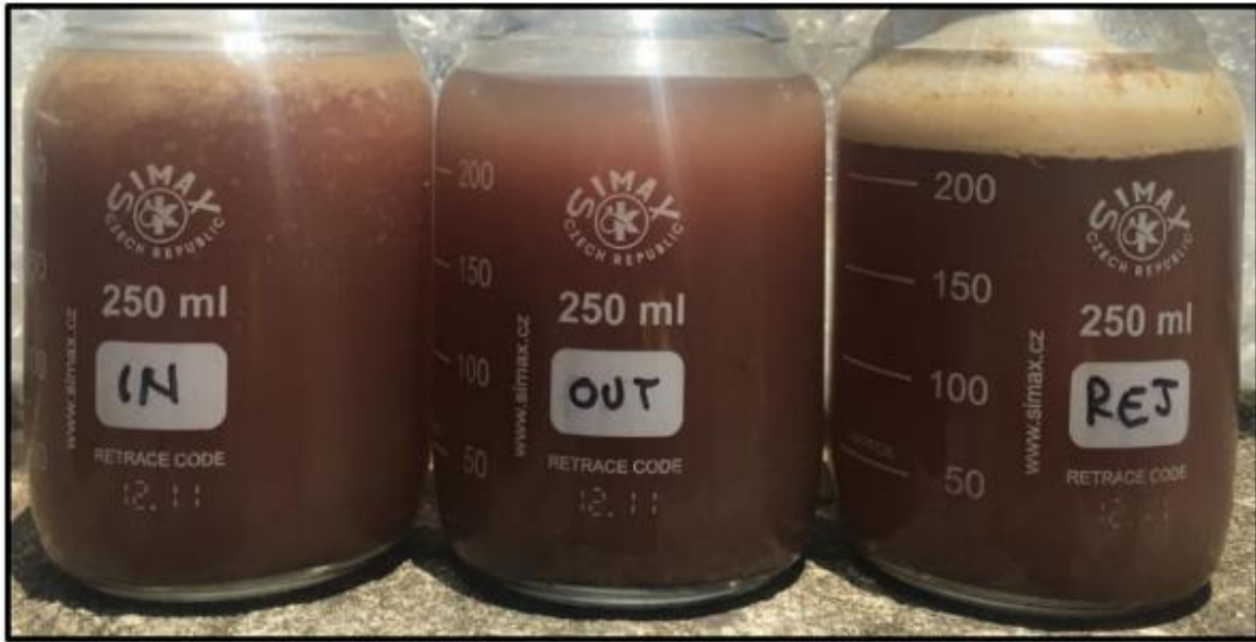
Figure 8: Visual results for hydrocyclone trial. From the left: red stream inlet (some fat collecting at the top), “water” out of the bottoms and the tops (or “reject”) with a clearly defined fat phase representing approximately 4.7% of the total tops volume.
