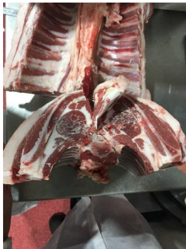
Result of chine off centre due to rolled product on infeed – Note the eye meat dimension
