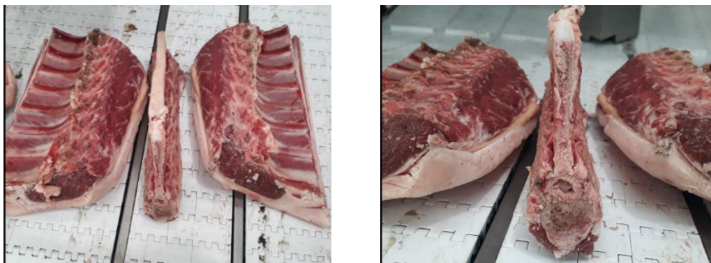
Figure 3-20 - Resulting cut remains consistent for the full length of the chine
