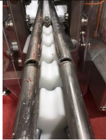
Infeed rails raised to attempt to support the product off the chain.
