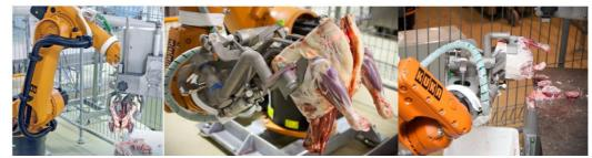
Figure 8: Robot holds shoulder primal, driving it against fixed blades to perform. de-boning (Scott Technology solution).
