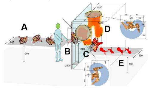
Figure 3: Early concept for an automated twin Robot Cell for lamb shoulder de-boning.
