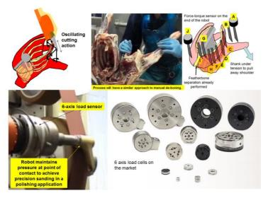
Figure 13: Force control using a 6-axis load cell on the robot tool flange.
