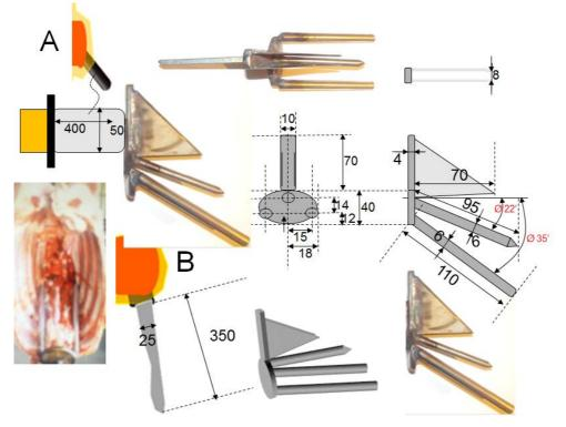
Figure 12: Fixation details, robotic tools and primal piece locating.
