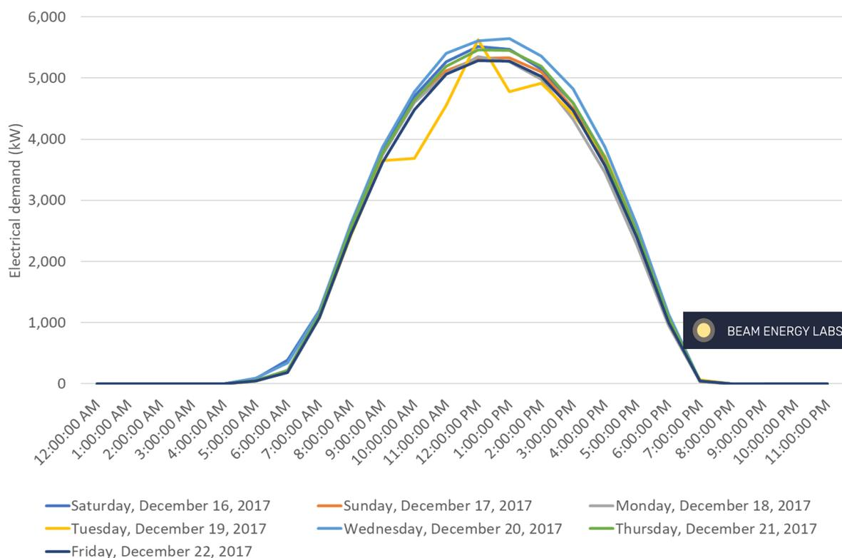
Figure 5: 7,000kWe solar PV generation profile during site peak demand, source: data extracted from Beam Energy Labs, commercial solar platform.
