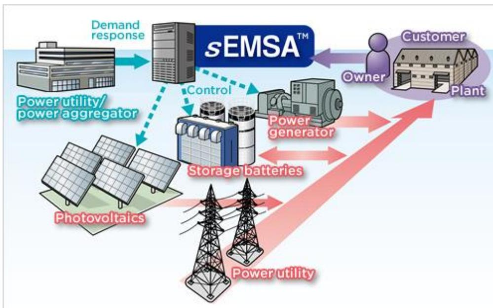
Figure 7: an infographic of interaction between grid, generation, storage and customer load, source <https://global-sei.com/products/semsa/>
