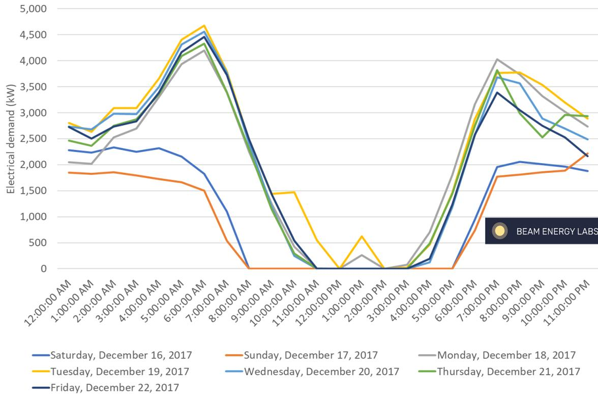
Figure 6: New site load profile with 7,000kW solar PV system
