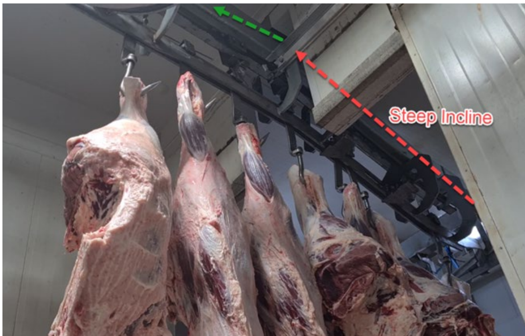
Figure 13: Annotated Infeed rail with Congestion of skids around the rail incline
