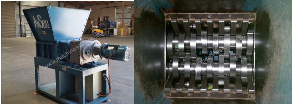
Figure 7: Example of a shredder for creating 20 mm particles from solid waste.
