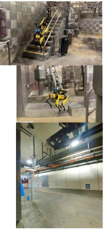
Improved access for robots into areas with sanitizing methods, allowing the robot to have a door open for it on arrival then walk through a wash bay that is safe for the robot but effective in sterilization.
