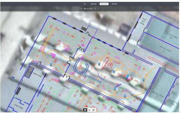
Figure 9 DroneDeploy's 360 Walkthroughs and Photos aligned to an aerial image with a Site overlay
