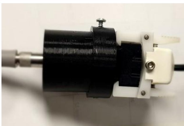
Figure 8: Prototype design of on-capillary fluorescence detector for detection of the labelled bacteria. Left is the prototype. Right is a schematic showing the optical configuration of the detector.
